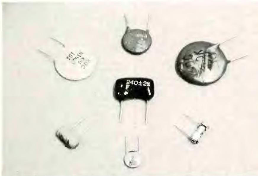
Six types of ceramic capacitors are grouped around a dipped-mica. Mica capacitors continue to be specified where stability and dependability are factors. Ceramic capacitors offer many different specifications.
