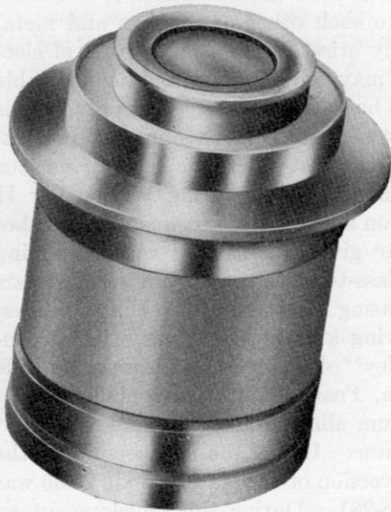
Fig. 16.1. Ceramic X-ray tube with a wide angle beryllium window for reproduction of Greuz Rays. Anode voltage 4 to 25 kv. Diameter of ceramic cylinder is 2 inch, over-all length 3\frac{1}{4} " 4 (Courtesy Machlett Laboratories, Inc.)
