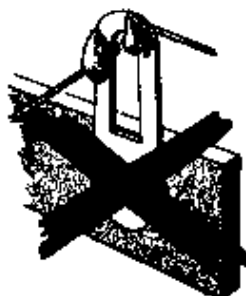
COLD SOLDER JOINT CONNECTION INSUFFICIENTLY HEATED
