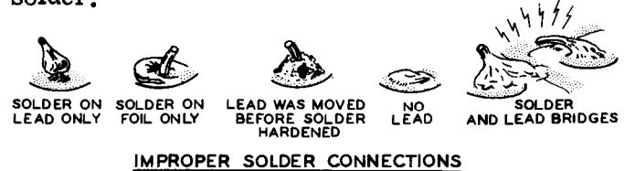
IMPROPER SOLDER CONNECTIONS
