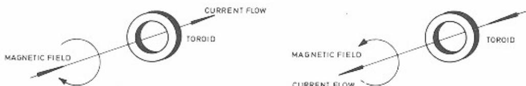
4 wires run through each toroid, 2 for write-in, 1 for read-out, 1 for trip.
