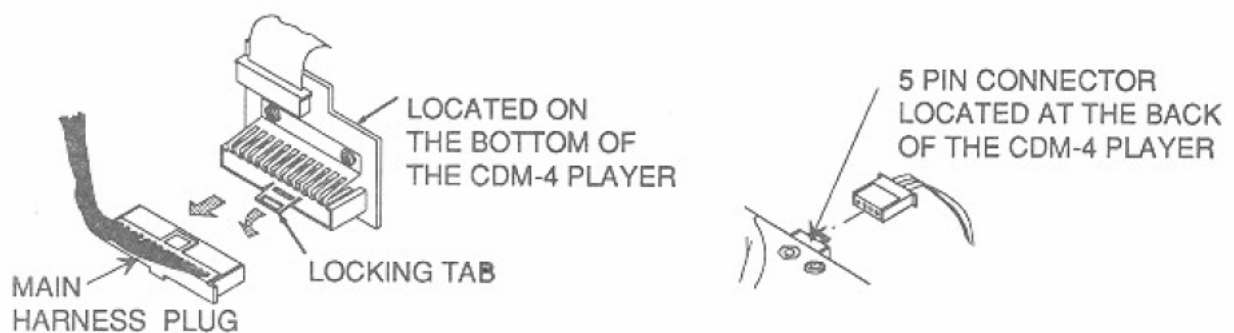
Figure 6-2B. Disconnecting The Main CD Player Harness
