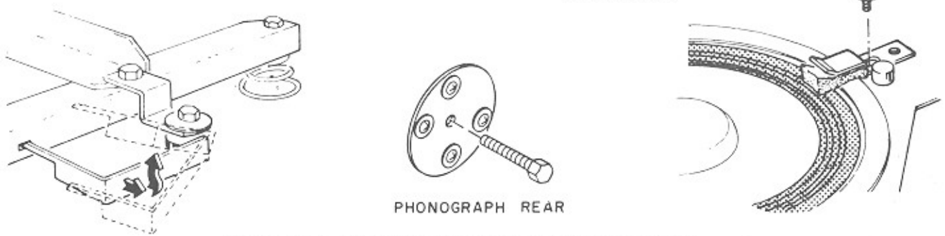
FIGURE 2-2. REMOVING MECHANISM TIE-DOWN BOLTS
