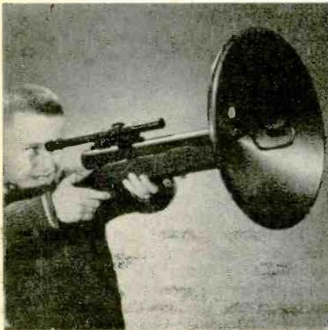
◀ **CORONA SPOTTER**—This Little League Eliot Ness is aiming a corona detector—not a gun—developed by Westinghouse. Corona from high-voltage lines, which wastes electricity and develops radio interference, may be spotted 75 feet away by aiming through the telescopic sight. Trigger turns on circuitry which makes corona static audible in speaker.
