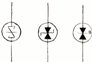
Electrical circuits, whether operated on a.c. or d.c. voltages, are often plagued by transient voltage peaks or surges, either externally or internally generated. Silicon and germanium semiconductor devices are especially sensitive to surge voltages, and a high-voltage transient or "spike" can destroy a semiconductor junction. Manufacturers have introduced special semiconductor devices to guard against and suppress transients. Most of these devices are made
