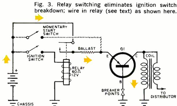
Fig. 3. Relay switching eliminates ignition switch breakdown; wire in relay (see text) as shown here.
