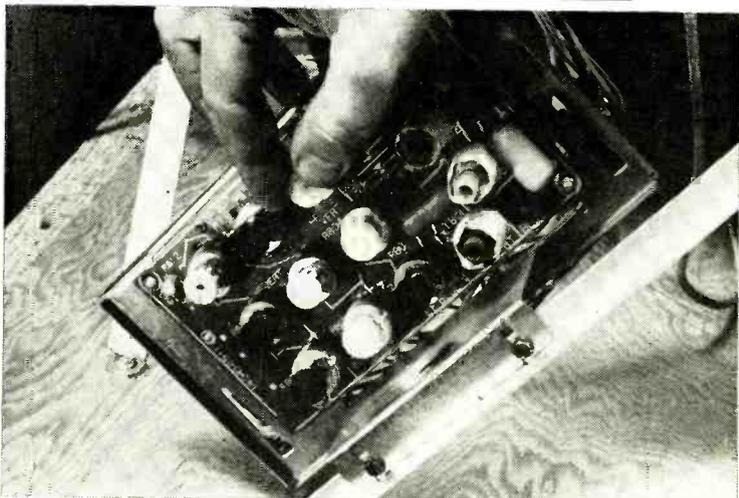
The kit builder works up the sound i.f. strip and the involved printed-circuit board containing the signal separating circuits for color reception. Point-to-point wiring to interconnect the three printed boards is simplified through the use of a supplied wiring harness with colored wire "breakouts" clearly identified.
