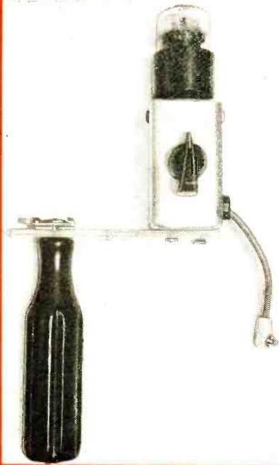
Mount the adapter on a bracket-mounted handle. Accessory shoe on bracket provides a convenient strobe base.
