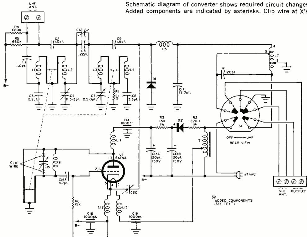
A twisted wire "gimmick" capacitor (*C15*) is connected to the tuner in the oscillator compartment. Clip these wires  $\frac{1}{2}$ " from the points at which they are soldered to the tuner. Do not disturb any other wiring in this compartment.
