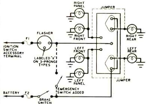
on when the brake pedal is pressed—an additional safety measure and one that is required by some new state laws. When the emergency switch is closed, all four front and back lights flash. In most cars, the jumpers simply tie together the two sets of wires at the distribution panel.
