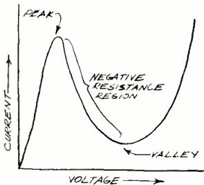
In a conventional semiconductor device, the current carriers move rather slowly, diffusing through the crystalline structure of the material. In a tunnel diode, the current carriers (electrons, for example) traverse the junction area at what appears to be the speed of light. In effect, when an electron enters the junction, another suddenly appears at the other side, much as if there were a "tunnel" through the junction area (hence the device's name).
