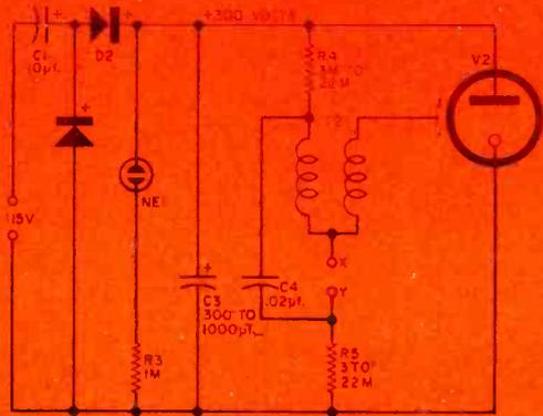
Schematic above shows typical strobe unit. At right is adapter unit.
