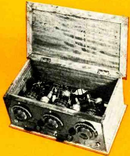
Popular Grebe Synchrophase of the early 20's used a two-step r.f. amplifier, detector, and two-step audio amplifier. Protruding from the polished panel are the three tuning dials with vernier dials below. Tubes were UV200's and UV201's powered by a filament storage battery, and dry cell B batteries. All wiring was done with spaghetti-covered bus bar.
