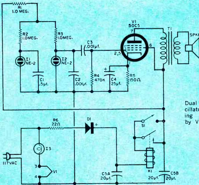
Dual neon lamp relaxation oscillator gives rising and falling siren effect. Amplified by V1, a 50C5, it is LOUD.
