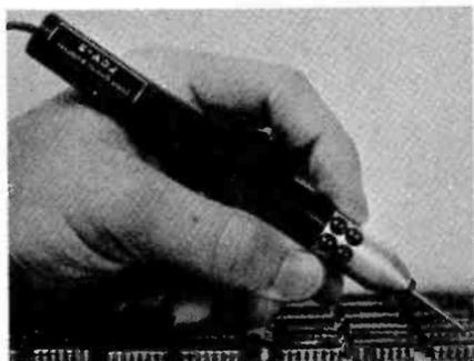
input. The LCA-2 is supplied with a 4-foot coaxial cable, BNC connector, and three input adapters. It can indicate polarity/duty cycle of pulse trains as high as 25 MHz. The probe measures 5½-in. long and ⅝-in. in diameter. \$69.50.
