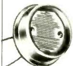
Cadmium sulfide photoresistor. 5 megohms in darkness to 100 ohms in bright light. 200 mW at 170V, maximum. 1/2" dia. x 1/4". 276-116 . . . . . 1.19
