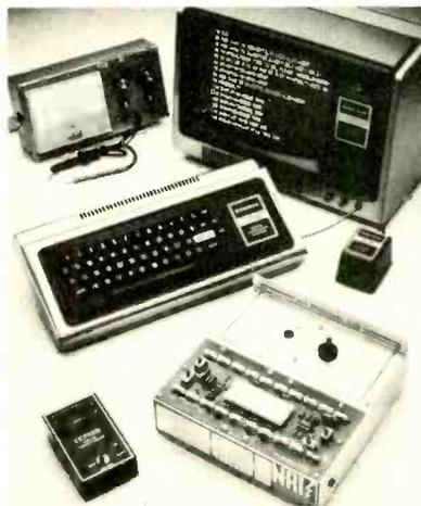
Training includes TRS-80 computer, transistorized volt-ohm meter, digital frequency counter, and the NRI Discovery Lab with hundreds of tests and experiments.
