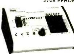
• 3 separate Output Registers & LED's for Hex, BCD entries, 16 LED's (27) for Data Register and 8 LED's for Data Memory Register. The Data Memory Register displays the content of the RAMs from the EPROM Chip.
