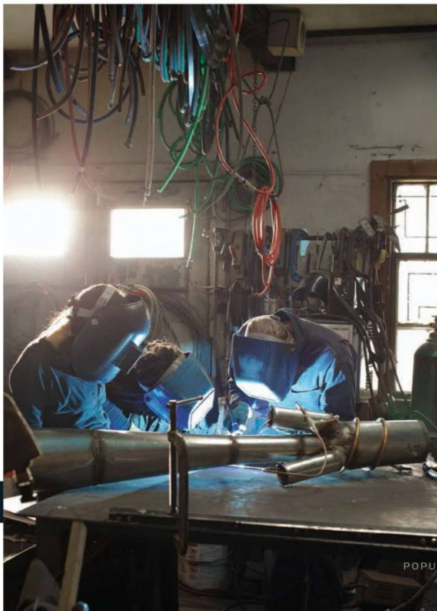
Top left: A pulse-jet-augmented motorcycle built by the Madagascar Institute. Left: The author takes the maiden flight of a fiery swing ride. Below: Madagascar members weld together a valveless pulse jet.
