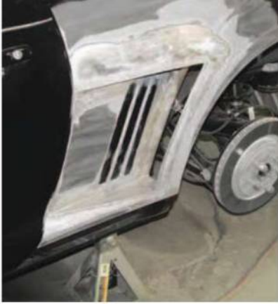
ABOVE: CUSTOM FABRICATED SIDE VENT
