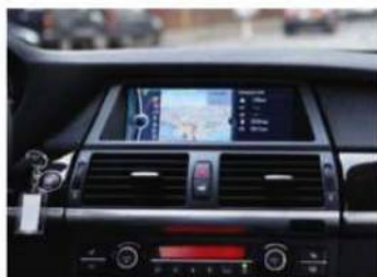
The X5's nav system uses GPS and a separate radio tuner to display Real Time Traffic Information (RTTI) and find the roads less traveled.
