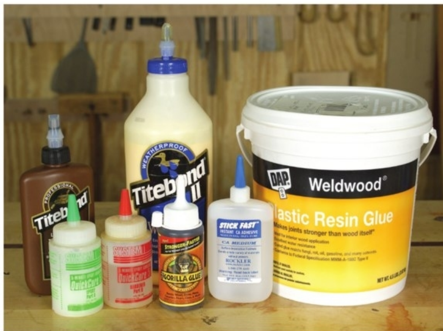
A glue for every reason. While woodworkers generally rely on yellow glue (polyvinyl acetate) for most glue jobs in the shop, depending on the task at hand, there might be a better choice available.
