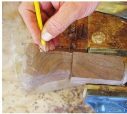
Layout begins. Mark out a flat area that's \frac{1}{8} " from the edge of the profile, then continue the line along the back edge of the foot matching the curve of the foot.
