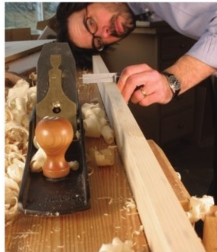
3 Joint and check. Dress your edge with a jointer plane, then use a square to confirm that your edge is true to one face of the board.
