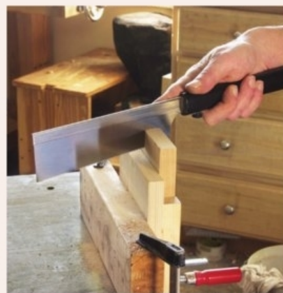
A good start. Many woodworkers start with a Japanese Dozuki as their first joinery saw. It is sharp, functional and doesn't cost a fortune.
