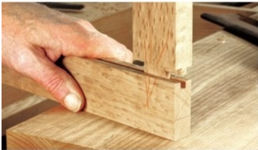
Double duty. The haunch fills the panel groove on the outer edges of the door. It also will keep the stile and rail faces aligned if the wood warps.
