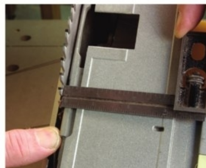
Properly set. A plunge-cut saw is set up with the blade slightly canted at the front. Here you can see the paper-thin gap needed to make a saw work its best.
