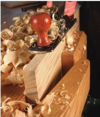
2 Rip with a plane. I use a scrub plane to work down to the line left by the panel gauge. Use short choppy strokes and each pass can remove 1/16 ". I reduced this board by 1" in width during one pop song on the radio.
