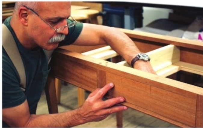
Made to fit. I fit the drawer front first, then build the drawer to match the front. My process is detailed in the February 2009 issue (#174) of Popular Woodworking .
