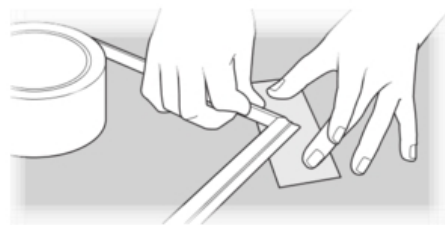
STEP 1: Press glued miters together on top of wide packing tape
