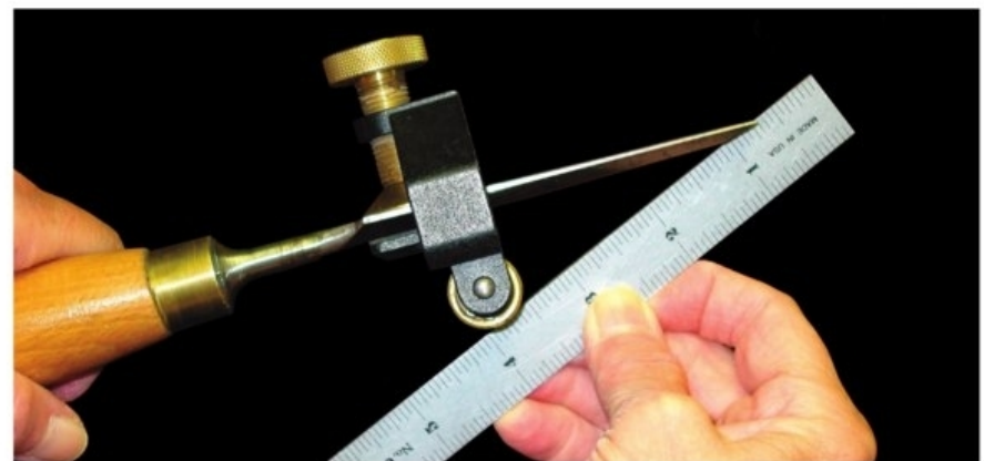
Adjust honing guide. The wheel and both edges of the hollow grind should all touch a straightedge to hone the desired angle.
