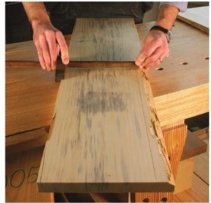
1 Gauge your width. I use a panel gauge to scribe the final width on my boards. Scribe the width on both faces of the board.
