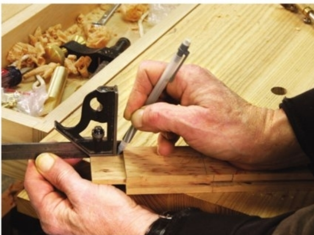
Easy transfer. Setting the end of the square's blade against the shoulder, and marking with a pencil at the bottom of the stock, transfers the depth of the groove to the haunch in the tenon.
