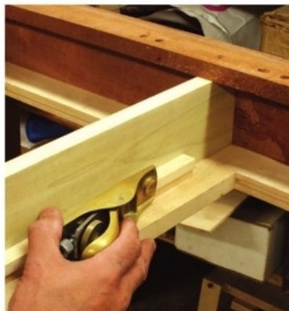
Planned to plane. The drawer runners are rabbeted underneath and cut short to allow me to reach in and plane them with my block plane.
