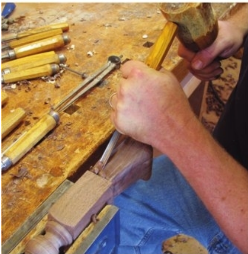
Time to carve. Use a #7 gouge to carve a shallow trough between the flat areas. Pay particular attention to those flat areas – try to keep a consistent width.
