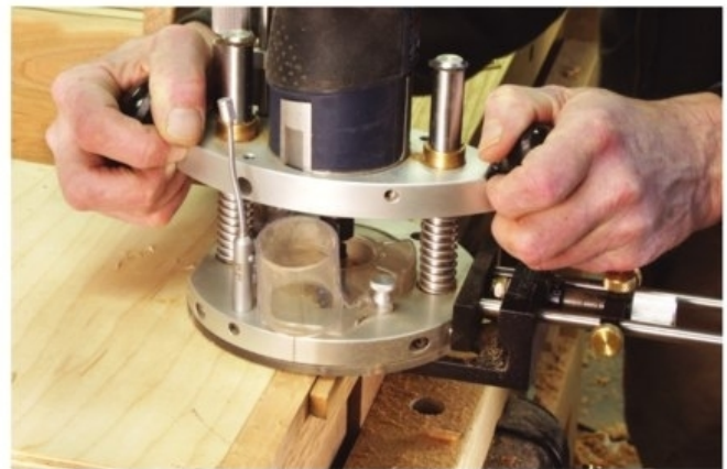
Support group. I clamp the door in my vise with the top edge of the door even with the top of a wood block. The fence on the router sets the distance for the hinge mortise, and the base of the router can't tip.
