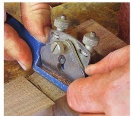
Straighten up. A spokeshave is quick to level and flatten any rough surface areas left from the band saw.
