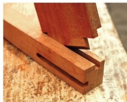
Long as I can. To maximize the length of the tennons in the rear legs, the ends are mitered.
