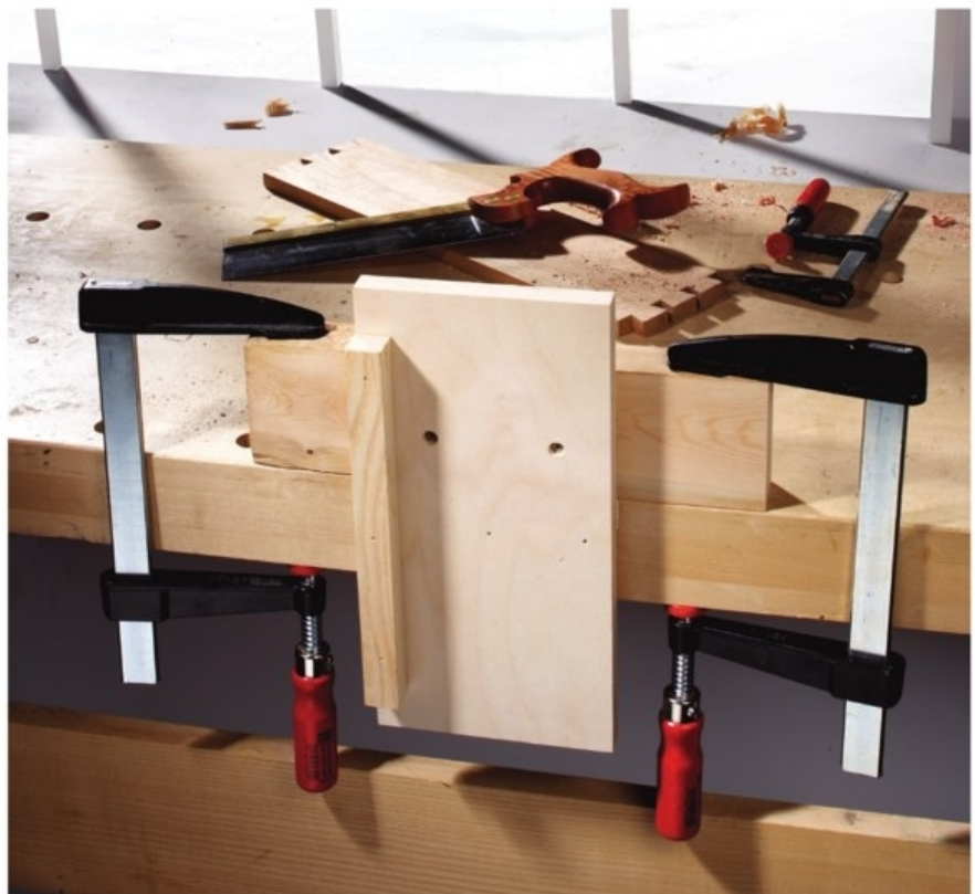
Simple solution. A vise is nice, but don't let the lack of one keep you from getting started with hand tools. This simple device will hold work vertically for cutting joints by hand.
