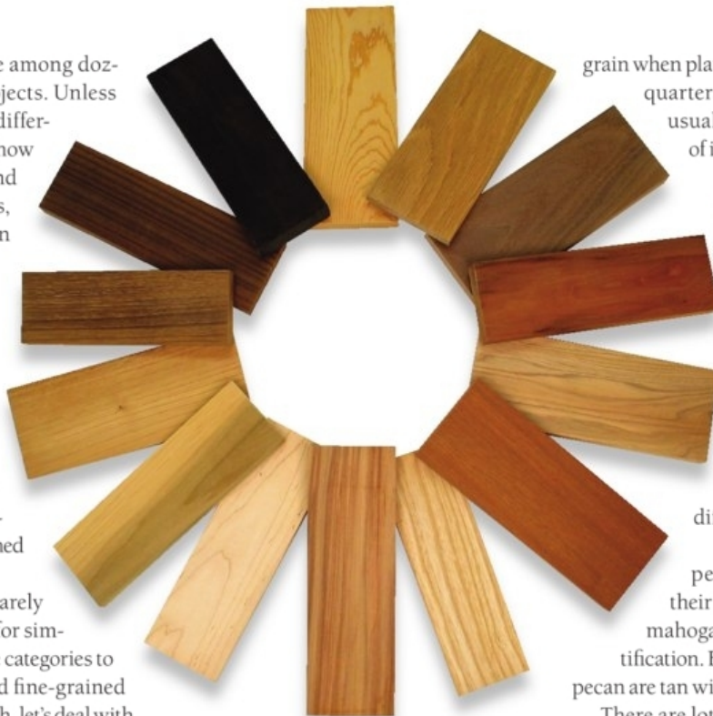
A fan of woods. Pictured are a number of woods woodworkers choose among for projects. Clockwise from the top are pine, oak, walnut, cherry, butternut, mahogany, ash, gum, soft maple, poplar, chestnut, teak, rosewood and ebony.
