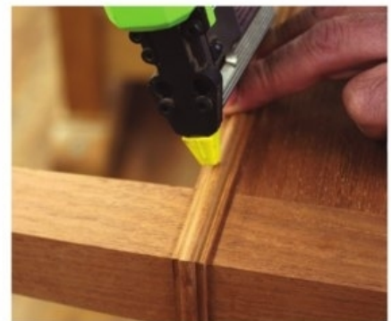
Finishing touch. The beaded trim is attached 1/8" above the bottom edge of the lower rails and aprons.
