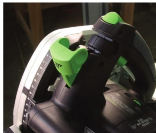
Quick-change artist. Festool's saw is by far the easiest on which to swap out blades. It's a one-handed operation.
