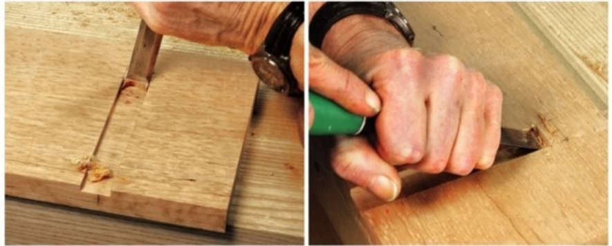
Finish by hand. A few cuts with a chisel complete the end of the dado for the top and bottom shelves. The front edge of the shelf is notched and ends 1/2" past the end of the dado. The notch is cut by hand with a dovetail saw.
