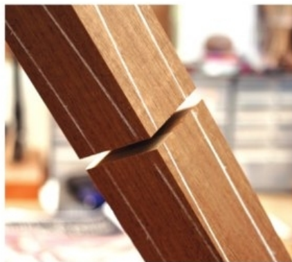
First things first. Before cutting the legs to shape, the dados for the bead are cut at the table saw. The dados on the back and inside are not as deep as on the front and outside.
