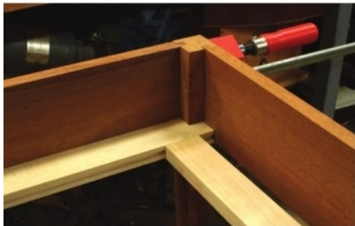
Loose fit. The front to back rails of the drawer frame are slid into the grooves, but not attached until the frame is glued inside the desk assembly.
