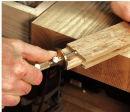
Dual-purpose tool. The cutter on the gauge removes the remaining material where the tenon cheek and shoulder meet. After scoring it with the gauge, pare with a chisel.
