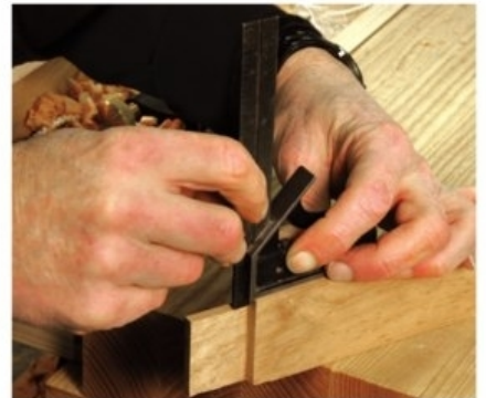
Drop-in measurement. With the adjustable square sitting on top of the groove in the stile, the blade is bottomed out to obtain the exact measurement for the depth of the groove.
