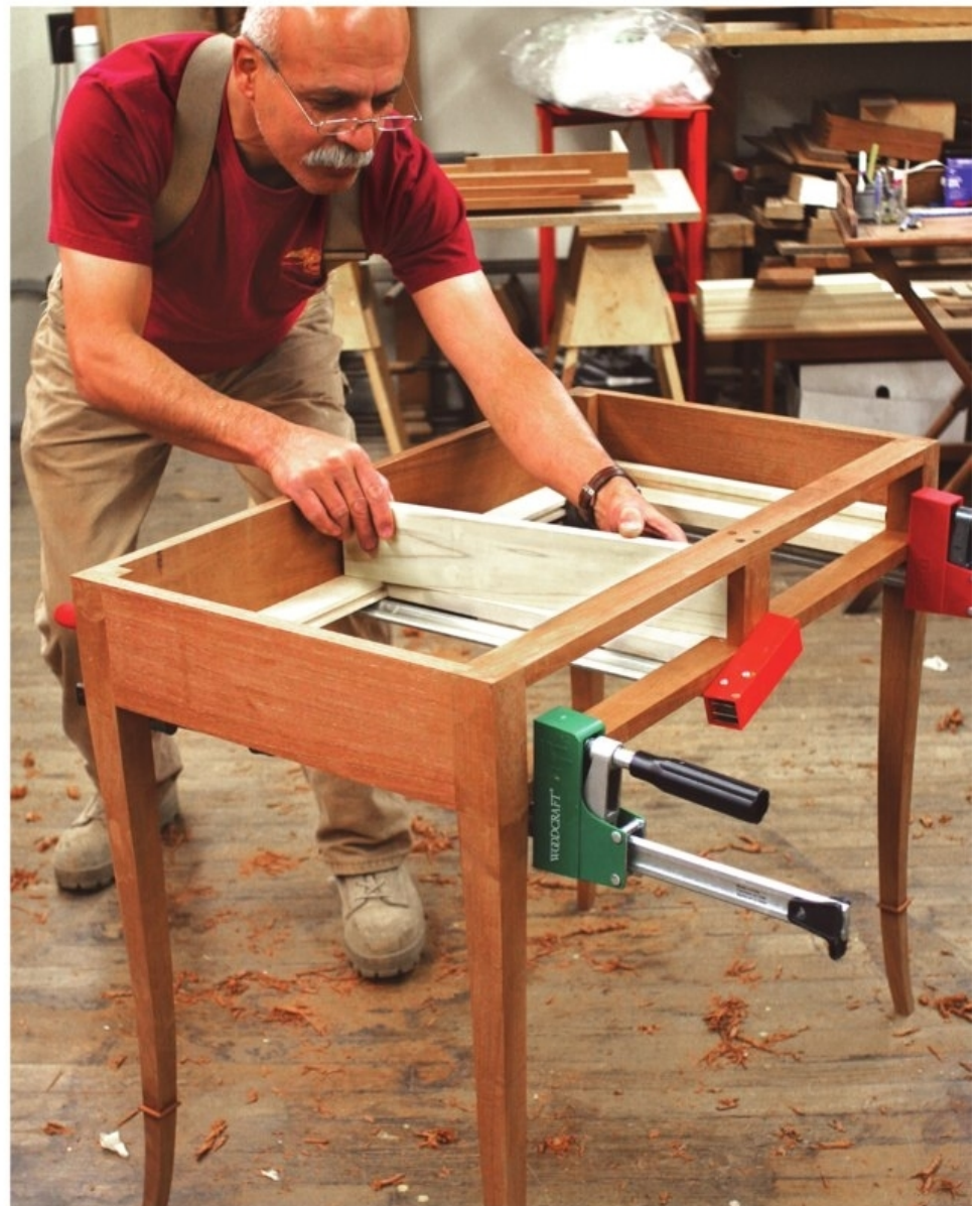
Divide and conquer. The drawer-front divider is slid between the rails and attached with screws. The partition is placed on top of the rail and behind the divider.
