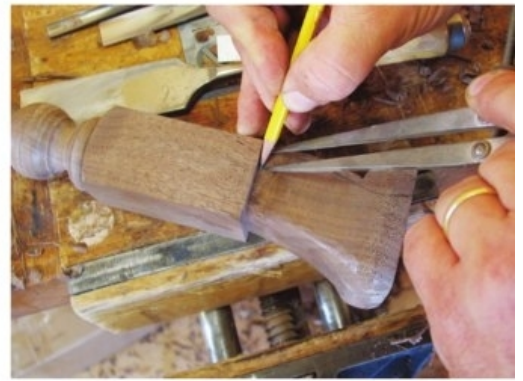
Divide and conquer. Use a pair of dividers to lay out the first fluted area; mark a flat area \frac{1}{8} " off the flute, then repeat. Extend the lines to the bottom of the foot, parallel to the outermost flat.
