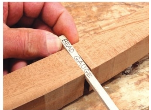
All things being equal. After shaping the leg, the dados should all be the same depth. I use a simple gauge block to check the dados and adjust as necessary.
