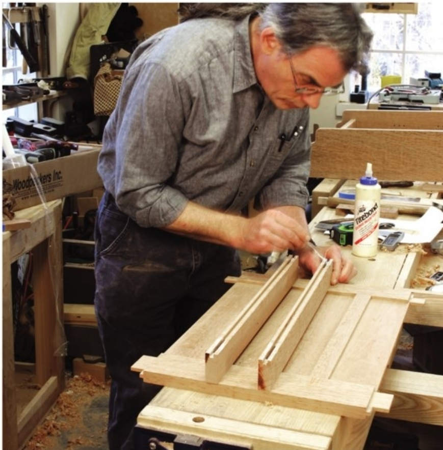
Two step glue-up. The center panel is put in place and the intermediate stiles glued between the top and bottom rails. After letting the glue cure, the outer panels are inserted, and the stiles are glued to the rail ends.
