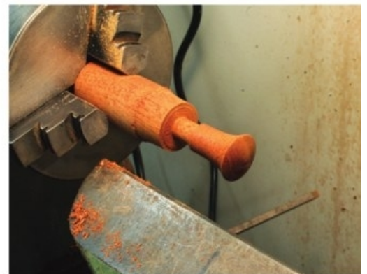
Start to finish. The knobs are turned in a three-jaw chuck. The tenon is formed, and the knobs are sanded and finished before being removed from the lathe.
