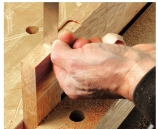
Final cuts. The router leaves a flat bottom and a straight back edge to the hinge mortise. The rounded corners, however, need to be removed with a chisel. Knifed-in layout lines provide a reference for the chisel.
