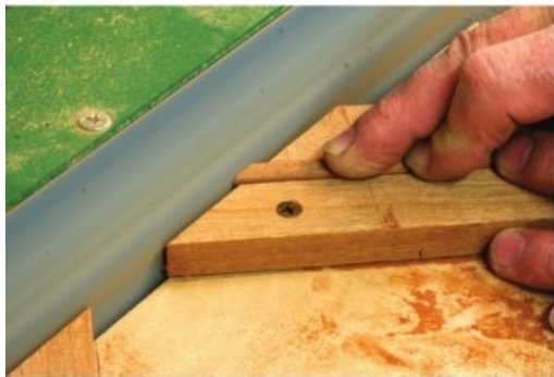
Too close for comfort. The beads on the legs are too small to miter with a power saw. I cut them by hand and created the miters on the horizontal belt sander.
