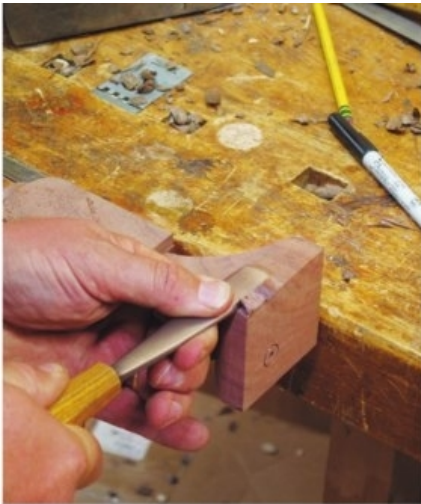
Round that toe. The cross-grain cutting action with a gouge leaves a clean toe area, but just rough in this curve. There's more carving to do.
