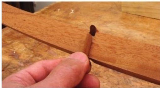
Off to a good start. Fitting the leg beads begins at the outside corner. This puts the easiest joint to fit in the most visible location.
