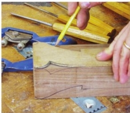
Best face forward. Once the foot blanks are sized and your pattern is drawn, transfer the profile onto two adjacent faces so the rear edges of the profiles meet at a corner.
