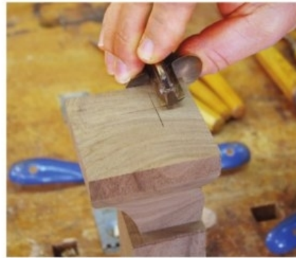
Set, mark and turn. Offsets in the design cause the turning center of the foot bottom to be shifted away from the foot front. A marking gauge set off the top center is the best method to locate this point.
