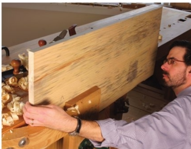
2 Rip with a plane. I use a scrub plane to work down to the line left by the panel gauge. Use short choppy strokes and each pass can remove 1/16 ". I reduced this board by 1" in width during one pop song on the radio.
