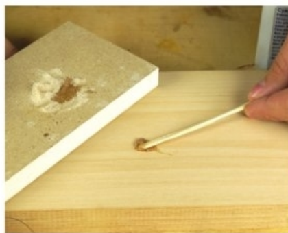
A fill-in filler. CA glue and sawdust make great homemade filler.
