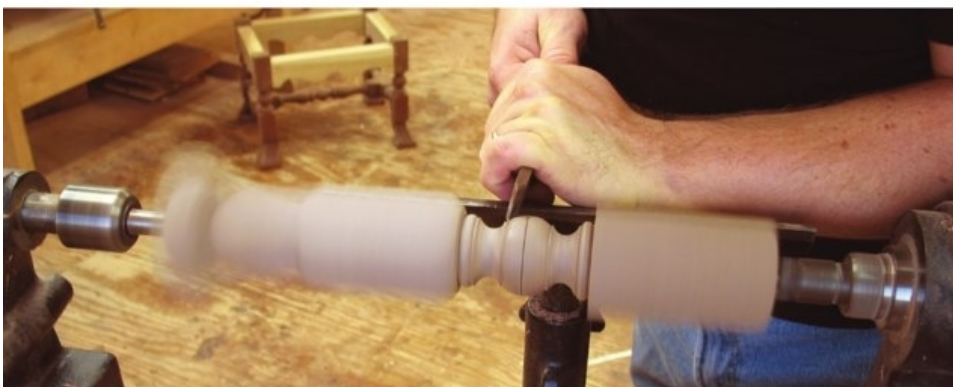
Transition details. The ring-and-ball design is very prominent in Pennsylvania furniture and adds a regional influence to the foot design.
