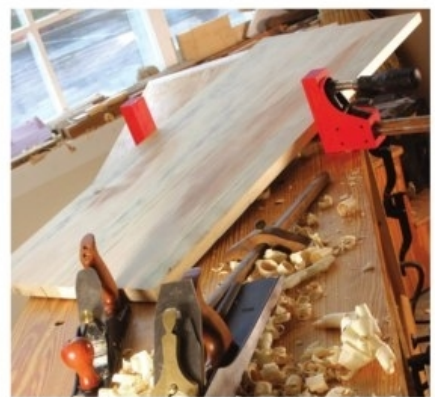
6 Results. With small panels (up to about 36" long) I can get away with using one clamp in the center. Larger panels will require clamps on the ends of the panel as well. PW
