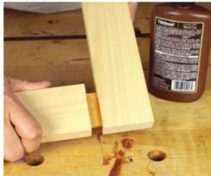
Best old glue. Hide glue is great for joints that are likely to need repair in the future.
