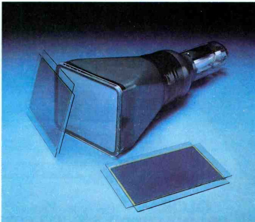
An LCD capable of replacing the CRT for oscilloscope applications has been developed by EEV. The display uses dye-phase-change technology, which eliminates viewing angle problems because no polarizers are required.
