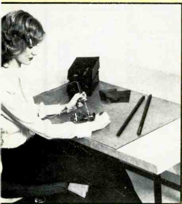
This conductive mat drains away static electricity before it can build up, preventing damage to sensitive ICs.
