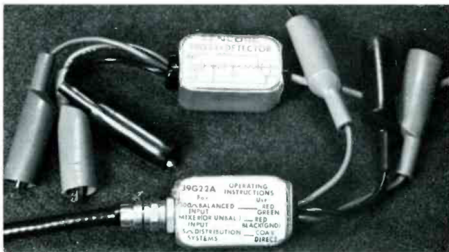
Fig. 1B The Sencore 39G23 Detector Probe and 39G22A Matching Pad are supplied with the generator.
