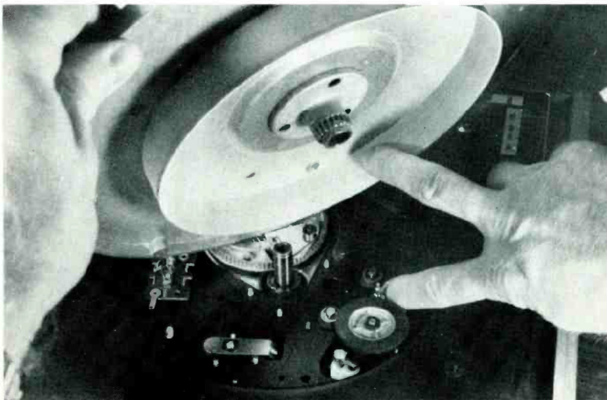
Fig. 1 Motor/drive system, showing (above) below-deck mounting of motor and drive shaft, and (below) idler above motorboard. Drive idler rotates against the turntable rim pointed out in bottom photo.
