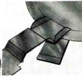
This tuner contact has been sprayed with an ordinary tuner cleaner. It looks clean, but close examination would reveal minute areas with corrosion and dirt.
