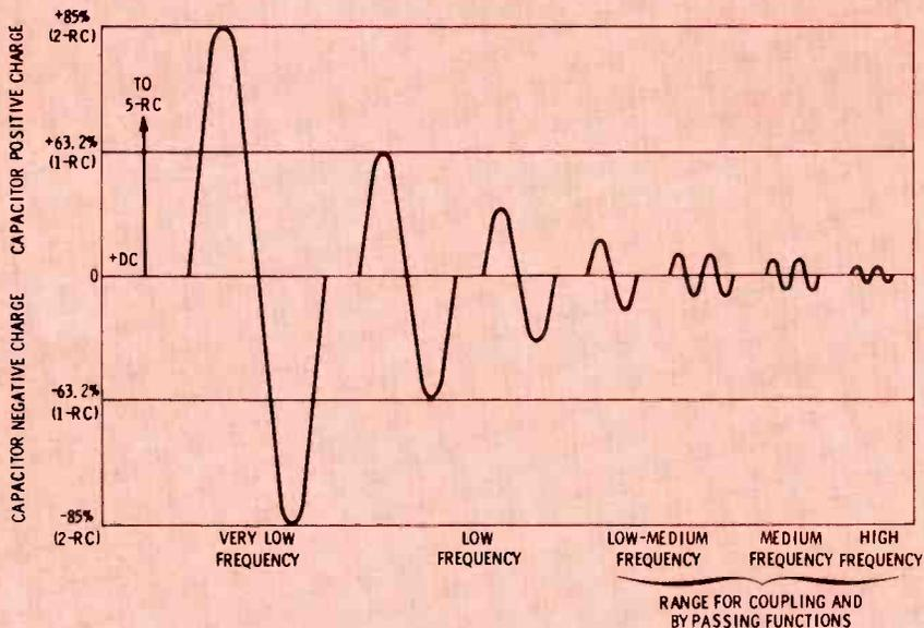
Fig. 3 If the supply voltage is changed to AC, the amount of charge the capacitor accepts is determined by the frequency of the AC.
