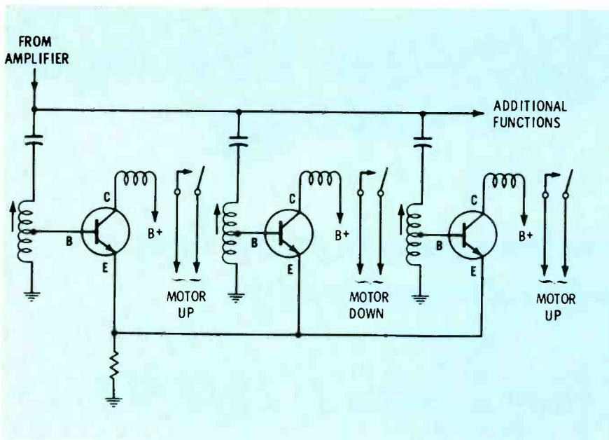
Fig. 5 Typical remote-receiver output circuits.
