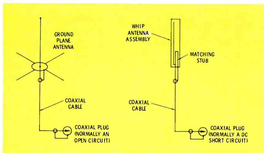
**Fig. 2** Whip antenna equipped with a matching stub normally indicates a dead short when checked with an ohmmeter; ground-plane type on left normally indicates an open circuit.
