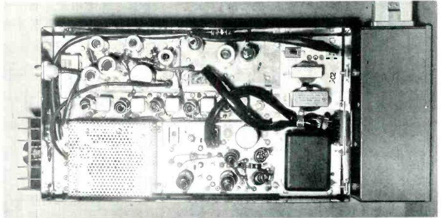
Example of a typical tube-type mobile communications unit.
