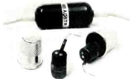
metal shields, the transformers come in two types: Model BV-16 is rated at 200 to 50K ohms and is mu-metal encased for chassis mount. Model BV-16E is electronically identical to Model BV-16 and comes encapsulated in vinyl, with an 8-inch length of microphone cable. Model BV-16E can be installed in or out of the microphone case, or it can be installed in the line.
