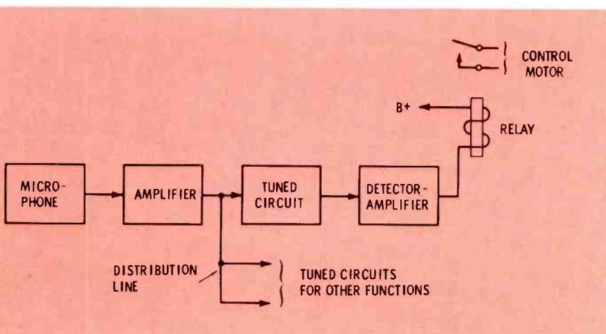
Fig. 4 Block diagram of a typical remote receiver.
