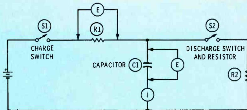
Fig. 2 (A) Schematic of the circuit used to chart the charge and discharge of capacitors.
