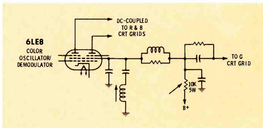
Fig. 3 Special tube oscillator/demodulator for color might fool you if you're not familiar with the stage. But that needn't keep you from tracing down DC trouble that puts a gray-scale symptom in the raster. Just start at the CRT and work back.
