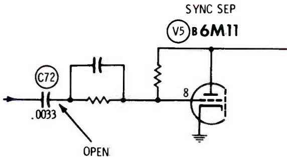
**Symptom**—Poor vertical locking and horizontal bending
