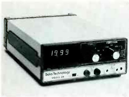
Model 20 has a resolution of 1 pf and an accuracy of 0.2% of reading for capacitance; four DC-voltage ranges with 1-mV resolution and 0.1% accuracy; four AC-voltage ranges with 1-mV resolution and 0.5% accuracy; and four resistance ranges with 1-ohm resolution and 0.2% accuracy. Other specifications include 3.5-watt power supply and 1/3-inch-high Sperry display.
