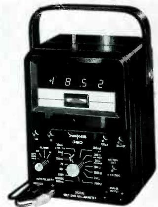
The new digital VOM features 29 AC, DC, and resistance ranges including low-power ohms. An analog output jack on the front panel makes it easy to interface with recorders and other instruments. Maximum full-scale response time to within rated accuracy is 2 seconds on DC, 5 seconds on AC. The unit operates from rechargeable batteries or AC line and may be operated while it is being charged.
