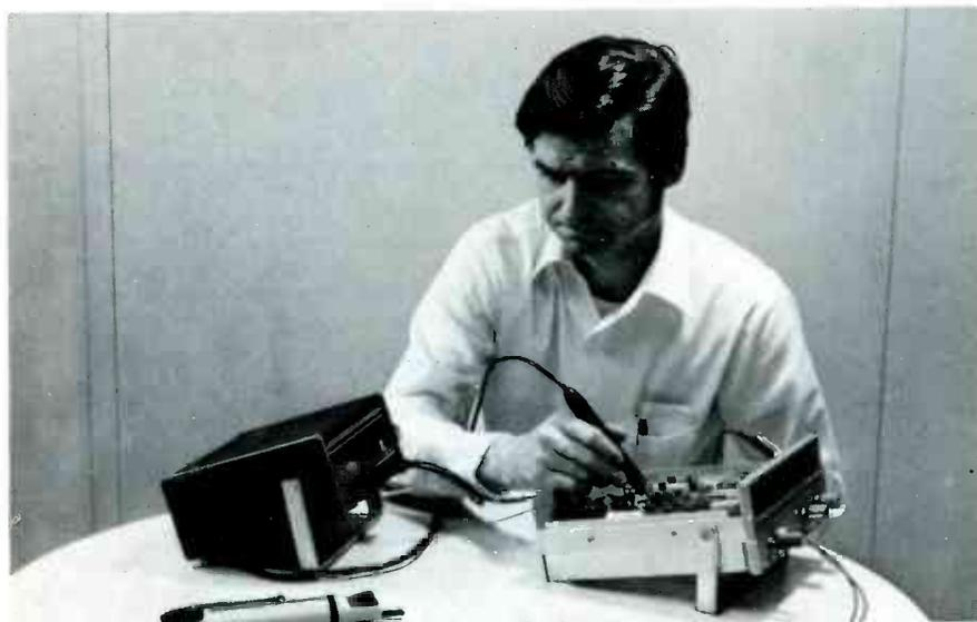
Fig. 1 Digital multimeters come in all sizes. One of our editors is shown using a B&K Model 281 to measure voltages in a Heathkit IM-102 which he built. On the table is a Model 970A Hewlett-Packard DMM, probably the smallest available.
