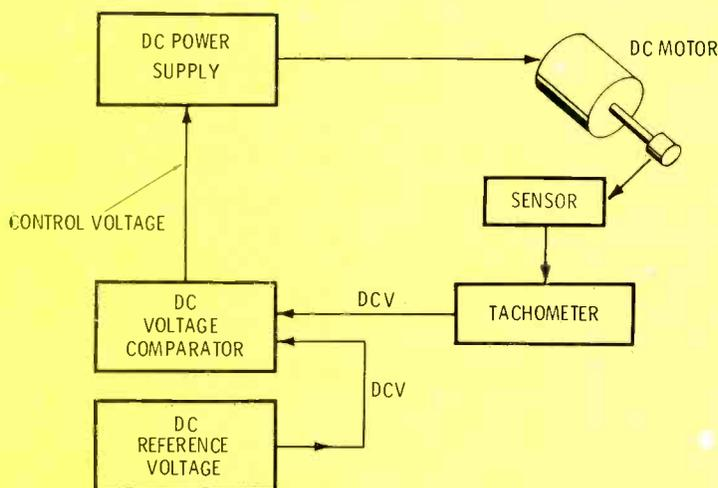
**Figure 11** A speed control for a DC motor is similar to the one in Figure 10, except the reference and sensor signals are DC, the comparator works from those DC voltages, and the motor speed is changed by varying the applied DC voltage.
