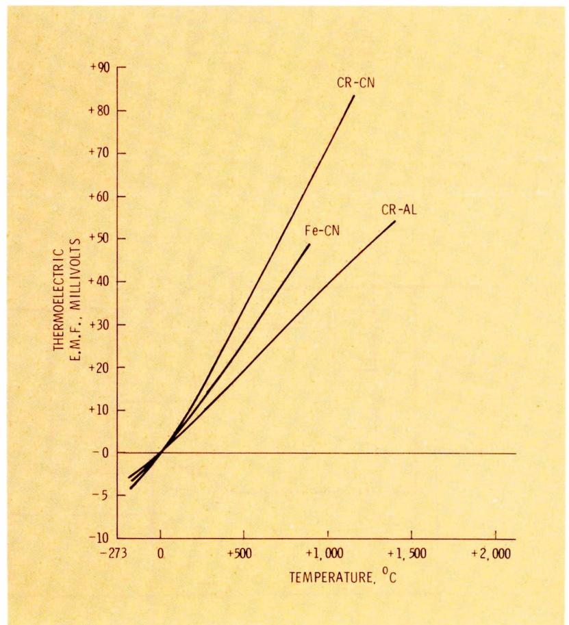
**Figure 5** These curves show the amount of millivolts produced by each junction of CR-CN, FE-CN, or CR-AL metals in a thermocouple.
