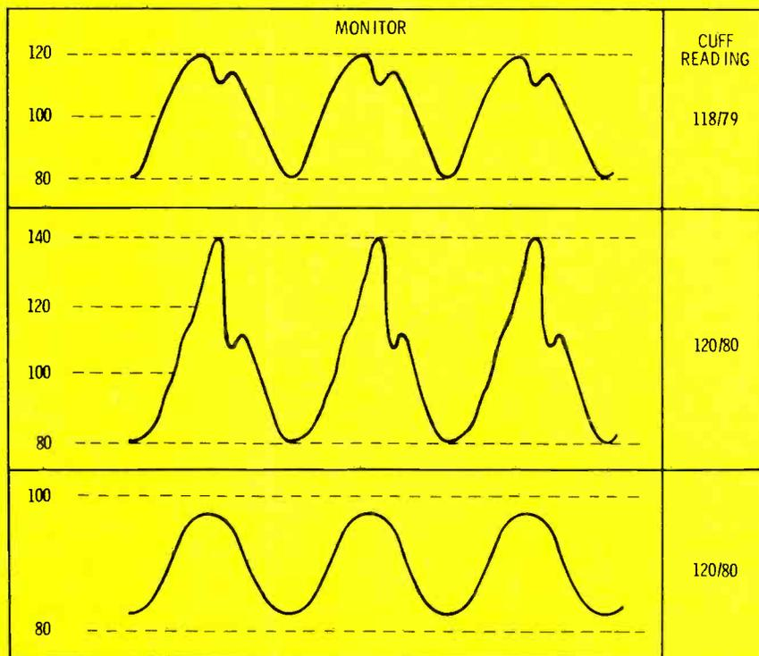
correct typical one for comparison. The effect of resonance (acoustic ringing) is shown in Figure 6B. If the catheter tubing finds resonances, then the rising edge of the waveform will tend to overshoot and ring. This is similar to the ringing of a tuned circuit in electronics. The cure for such ringing is to change the diameter of the tubing, the length, or the type of tubing. Another possibility is to reposition the catheter.
