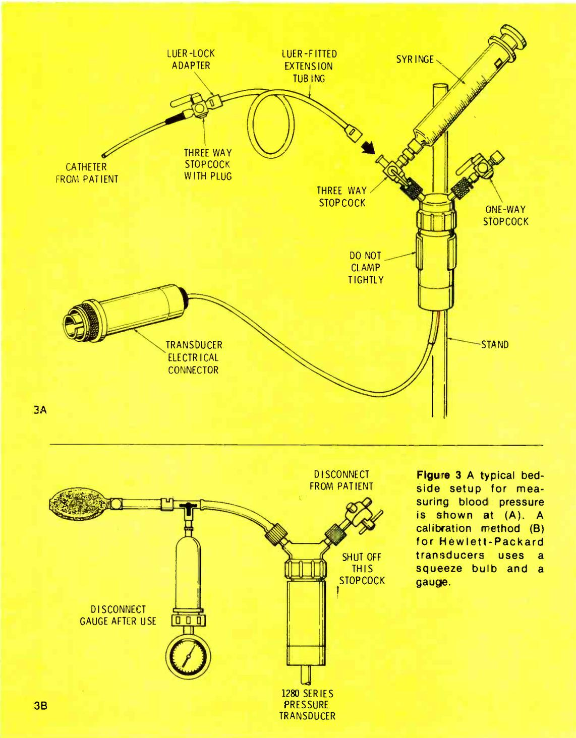
**Figure 3** A typical bedside setup for measuring blood pressure is shown at (A). A calibration method (B) for Hewlett-Packard transducers uses a squeeze bulb and a gauge.
