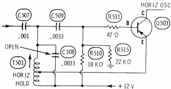
**Symptom**—Incorrect horizontal frequency, width is narrow
