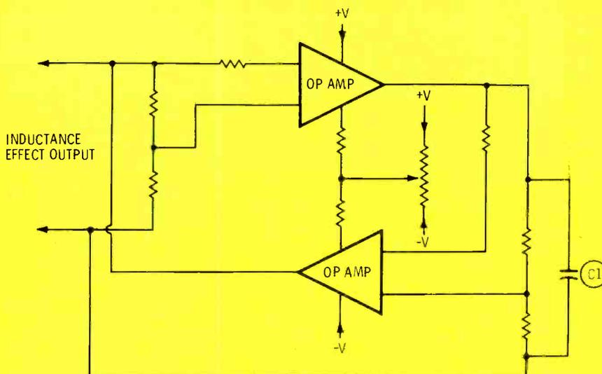
**Figure 3** An inductance effect can be obtained by this circuit that uses op-amps. The advantage over discrete coils is that such **gyrator** circuits can be made small enough to be included inside ICs.
