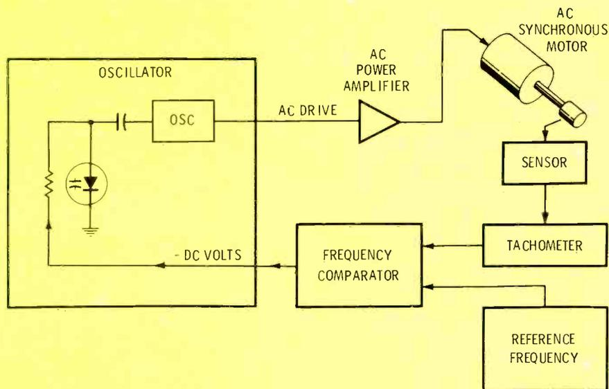
**Figure 10** One type of speed control for a synchronous motor uses a closed-loop, and compares the tachometer reading of the motor speed against the reference frequency. Varying the frequency of the motor voltage changes the motor speed.
