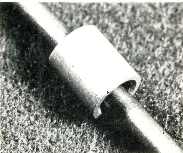
**Figure 4** When placed around wire conductor, ferrite beads act as a small inductance. The advantage over coils is that the wire and bead do not have any self-resonance.
