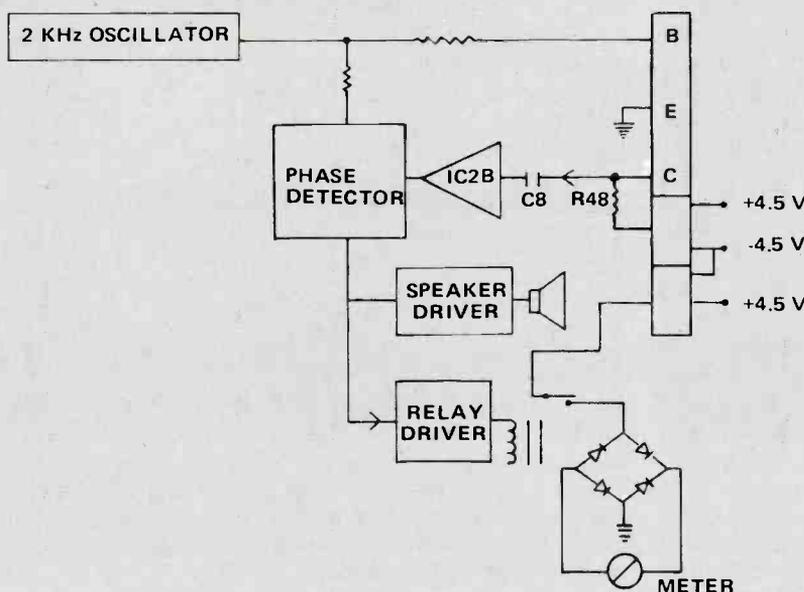
Figure 1 After the permutator switch has been set correctly, a 2-KHz square-wave signal is fed to the base of the transistor (that's being tested), and bias of the proper polarity is applied to the emitter. A sample of the base signal, and a sample of the inverted square waves from the collector, go to a logic phase detector. When both signals are present, the meter and the speaker tone are activated. (Courtesy of Sencore)
