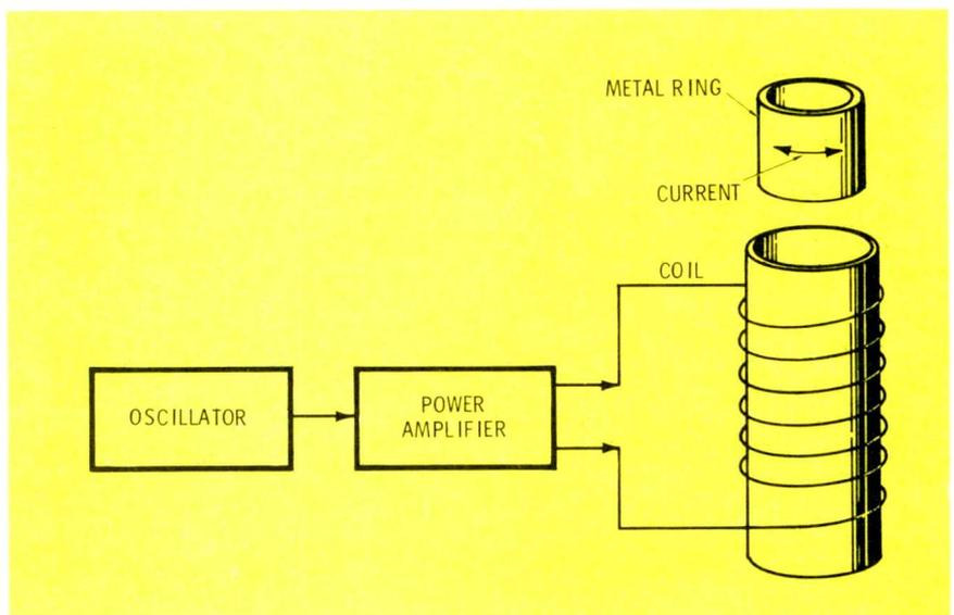
**Figure 1** AC current in a metal ring placed in the field of an inductor produces heat. The RF frequency and the amount of power applied to the coil determines how hot the ring becomes. •
