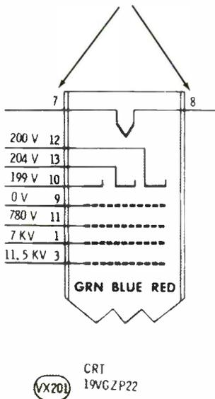
If the problem occurs slowly, a possible cause could be cold solder joints at the heater circuit of the CRT in the 9-121 video output module that's mounted on the base socket itself.
