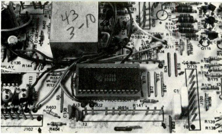
IC103, the control processor, is the largest one on the control chassis. It has 28 pins. Three of the ICs incorporate the new Integrated Injection Logic (called I squared L) that permits low-current drives; therefore, the "highs" are supplied at lower DC voltage levels than for other digital circuits.
