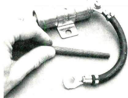
**Figure 5** A round file or tapered reamer should be used to enlarge the mounting hole or terminal hole, as needed.
