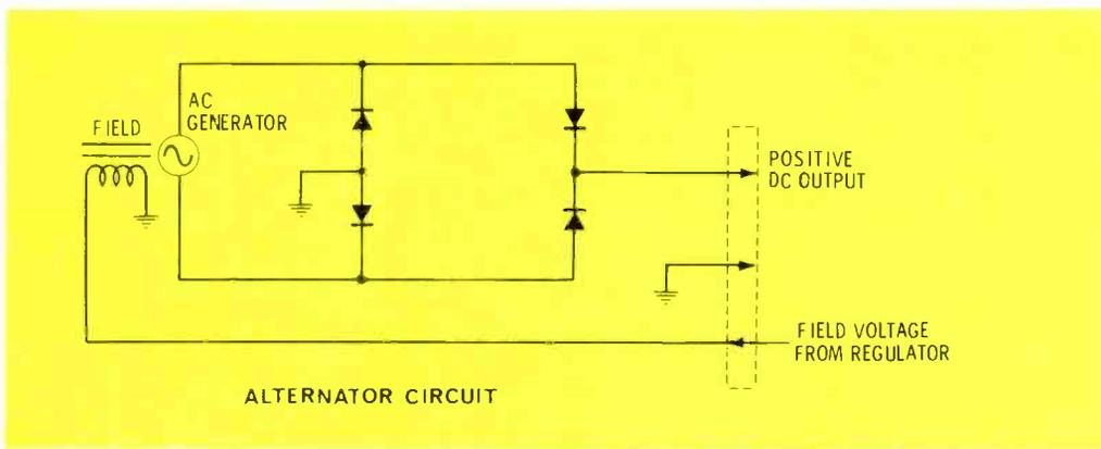
Figure 1 Alternators produce AC voltage, which is rectified by diodes. Noise sources include the slip-rings and brushes that feed power to the diodes, and the diodes themselves. Not all have the negative side grounded.
