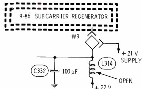
**Symptom**—Retrace lines, little control of brightness, and the video is negative
