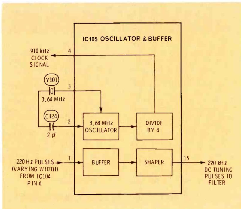
Figure 8 IC105 has two separate functions. It is the 3.64-MHz oscillator and X4 divider; also, a section acts as a buffer and waveform shaper of the 220-Hz pulses that will become the tuning voltage.
