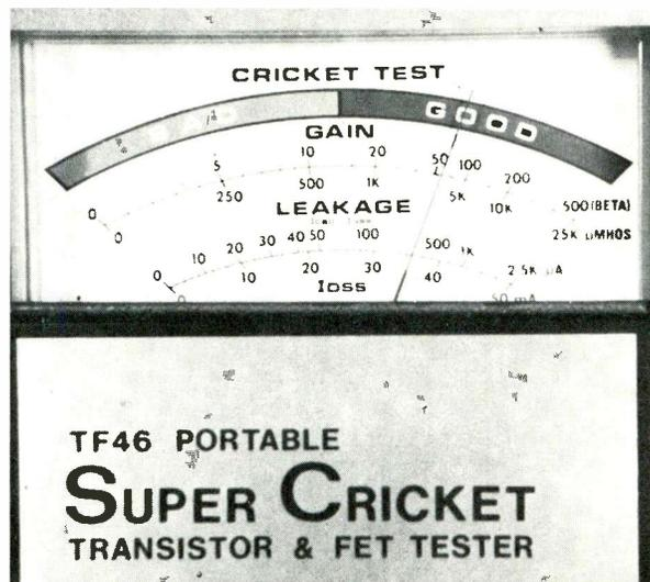
Figure 3 The five scales of the TF46 meter are, from top to bottom: good/bad Cricket and battery test; 0 to 500 beta for bipolar transistors; 0 to 25K microhms for FETs; 0 to 2,500 microamperes for transistor leakage; and 0 to 50 milliamperes for FET leakage.
