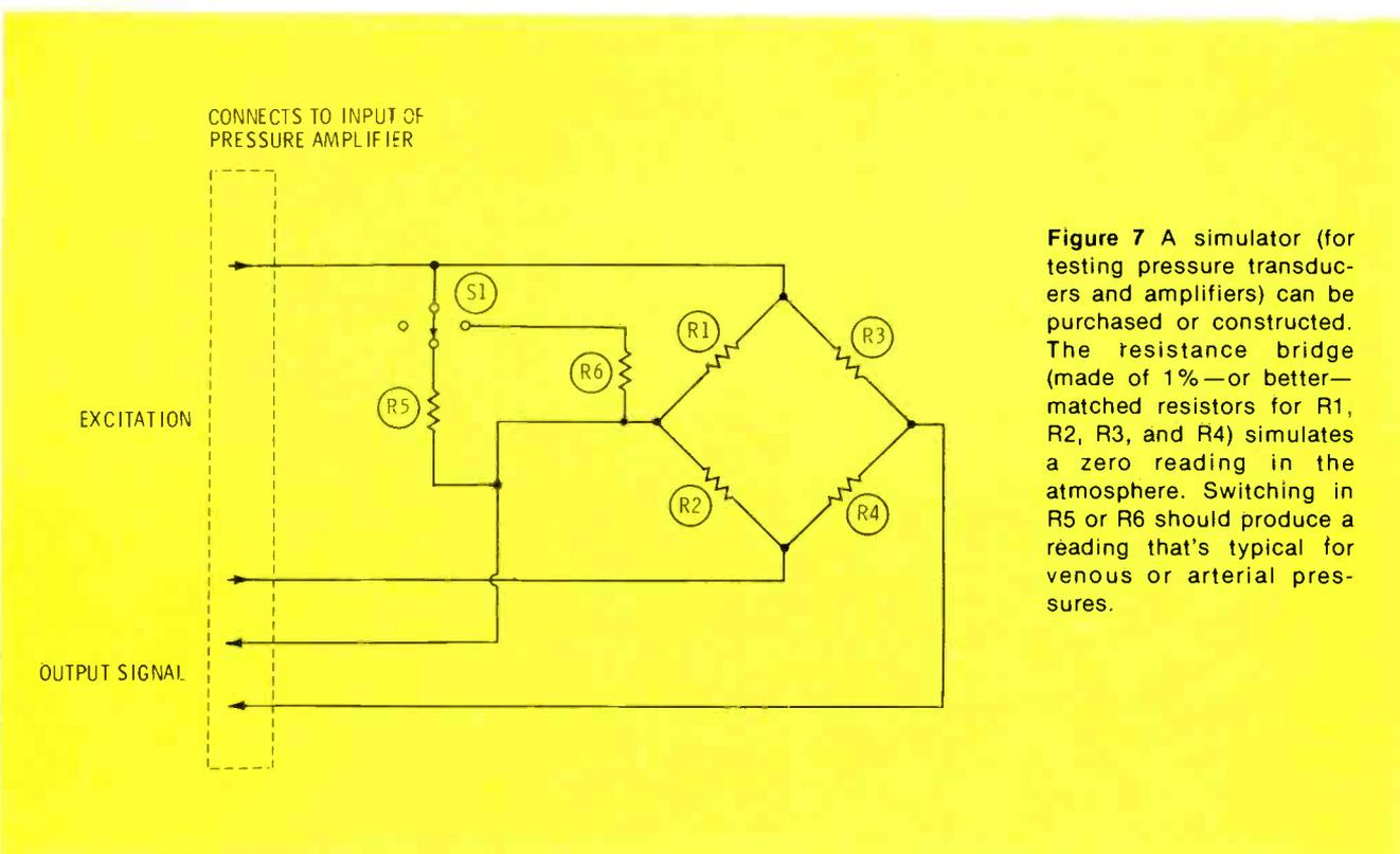
**Figure 7** A simulator (for testing pressure transducers and amplifiers) can be purchased or constructed. The resistance bridge (made of 1%—or better—matched resistors for R1, R2, R3, and R4) simulates a zero reading in the atmosphere. Switching in R5 or R6 should produce a reading that's typical for venous or arterial pressures.
