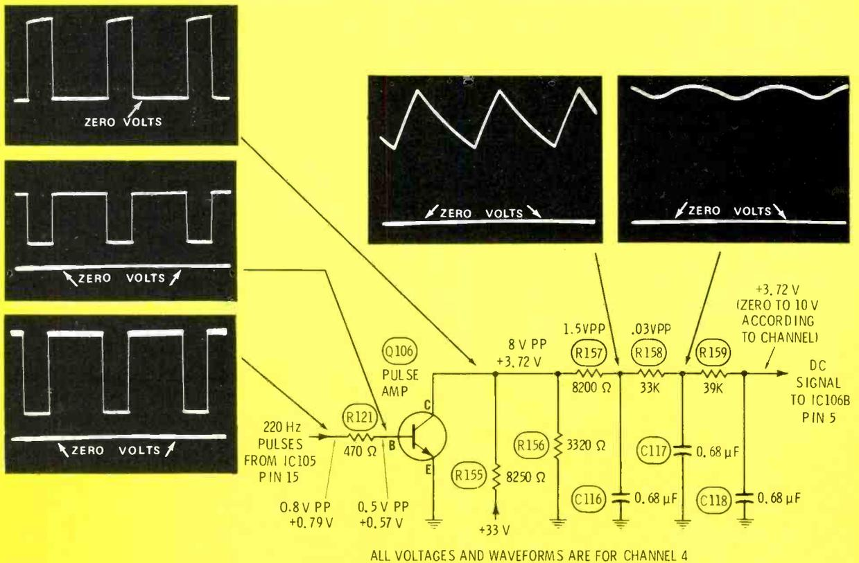
**Figure 9** Q106 amplifies and inverts the varying-width pulses. The waveforms, DC readings, and AC peak-to-peak readings were recorded for channel 4, and they will be different for other channels. Output from R159/C118 contained so little ripple that it could not be seen on a sensitive scope. After mixing
