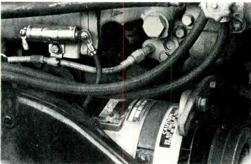
Figure 3 Mounting the coaxial capacitor on the engine block is not best, because of the extra heat there. On the other hand, you should mount the capacitor as close to the alternator as possible. Ideally, the capacitor should be mounted on the alternator or its bracket.
