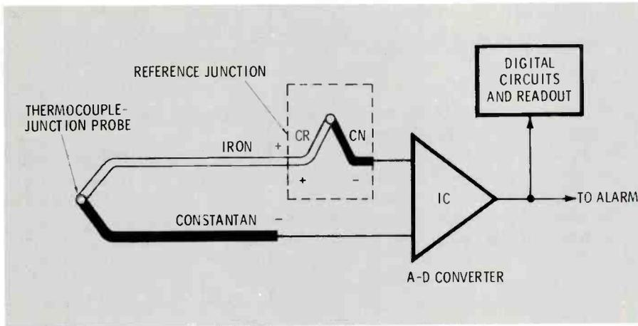
Figure 6 Accurate temperature measurements by a thermocouple device requires a reference junction, operated at the ambient temperature, that opposes the voltage from the measuring junction. The output can be increased by using multiple junctions. An analog meter can be used to read the output voltage, or (as shown) a digital circuit can activate an alarm and show the temperature on a decimal readout.
