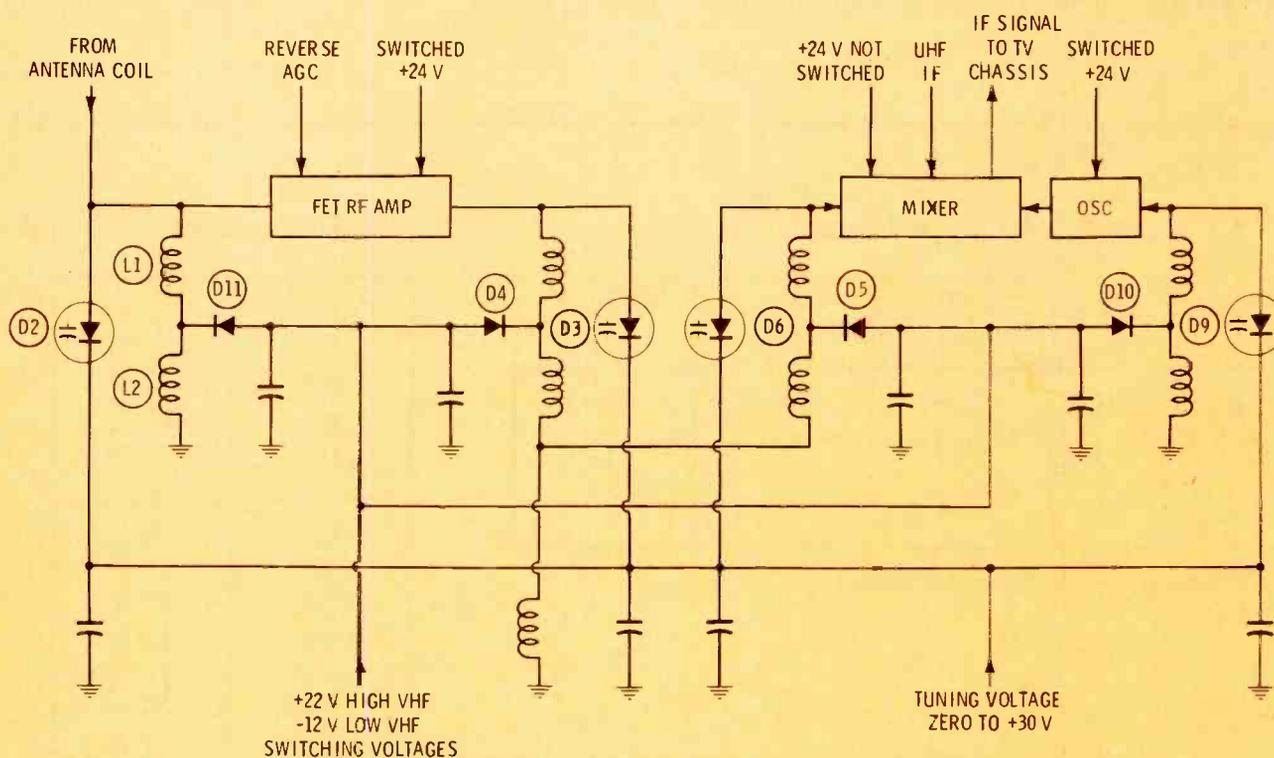
Figure 2 A block diagram of the Voltage-Variable Capacitance (VVC) VHF tuner shows the tuning varactors (D2, D3, D6, and D9), and the switching diodes (D11, D4, D5, and D10). L1 is the high-VHF RF coil, and L2 plus L1 is used to tune the low-VHF band. Therefore, for low-VHF operation, about -12 volts is
