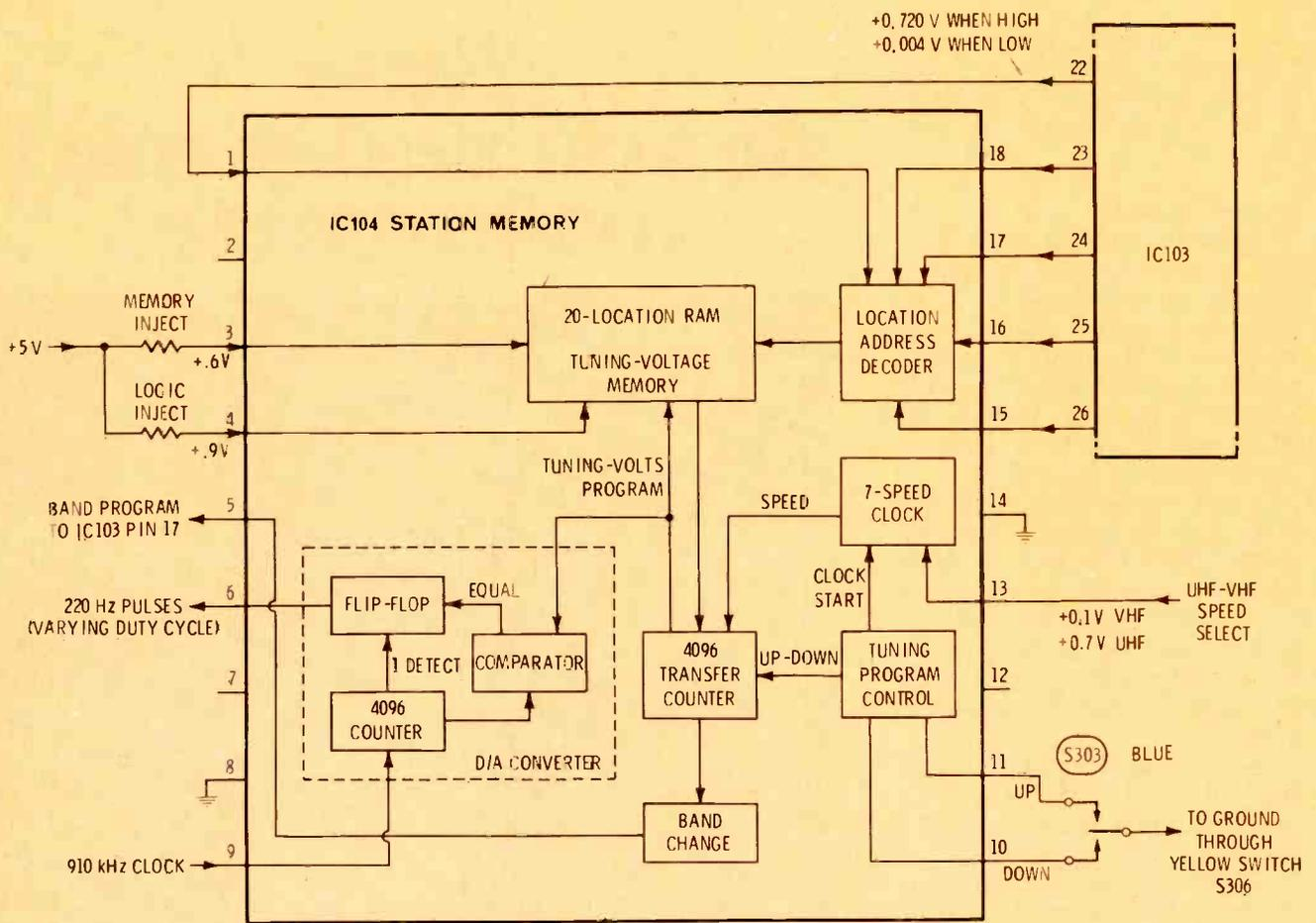
Figure 7 Internal functions of IC104 are shown by the blocks, with pin numbers in the proper sequence. The varying-width pulses of DC voltage from pin 6 are filtered
