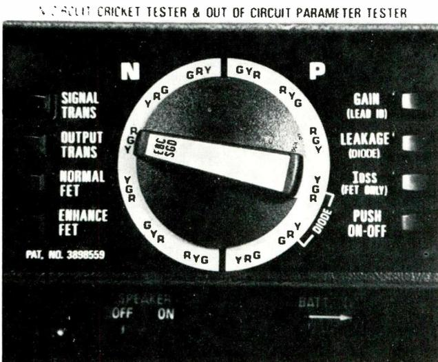
Figure 2 In the center is the permutator-switch pointer, which selects all combinations of leads and polarity. The eight pushbuttons at the sides select the conditions and functions. The gain, IDSS, and leakage buttons are the only ones that do not latch. The SPEAKER OFF/ON switch can be seen dimly at the left bottom; it is at the back of the storage compartment. The BATT TEST switch is shown at the right bottom corner.
