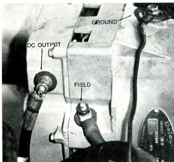
**Figure 4** Here are examples of different alternators, showing the terminal posts and the ground. NEVER connect a capacitor to a field wire or post. Connect it only to the DC-output post.
