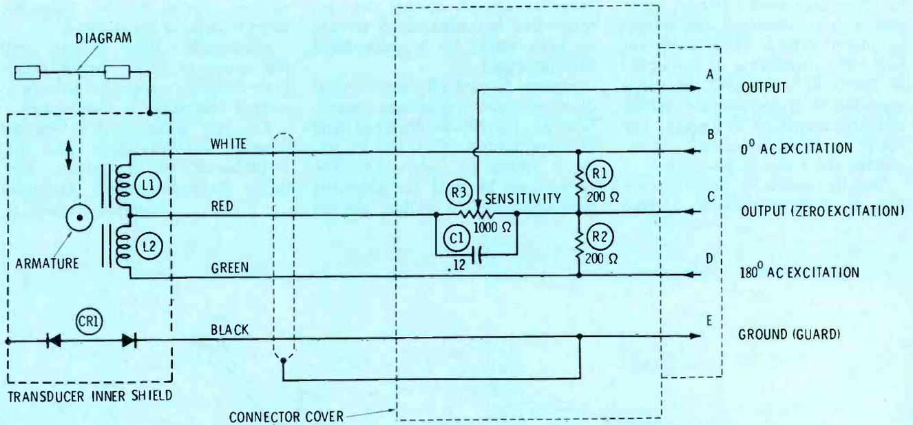
**Figure 4** This is the internal circuit of Hewlett-Packard 1280-series blood-pressure transducers. The three resistors are mounted inside the large connector. Included is a graph of pressure versus output voltage.
