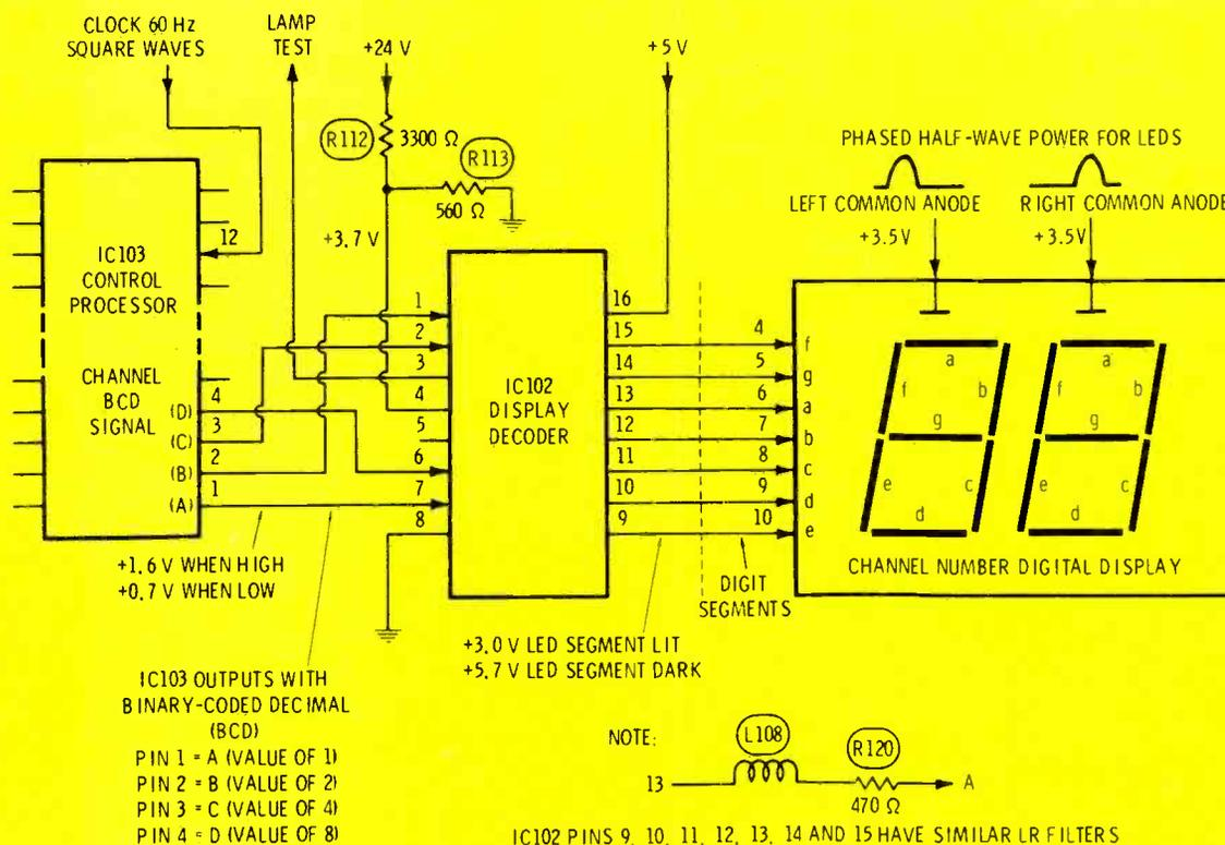
**Figure 6** The display decoder, IC102, receives the A, B, C, and D lines of the BCD output from IC103 and changes the BCD to the logic required for lighting the seven-segment LED display. Multiplexing of the two channel digits is done
