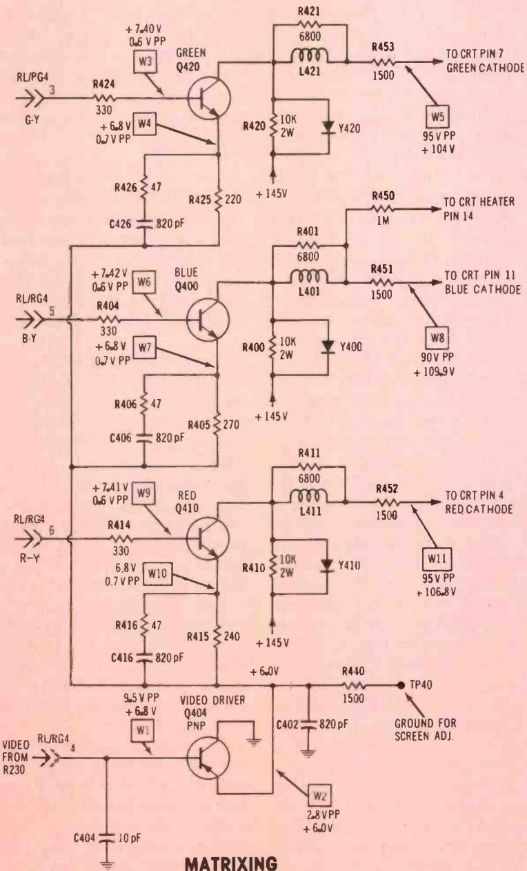
Figure 9 Luminance video and demodulated chroma signals are matrixed inside Q420, Q400 and Q410. Chroma signals are applied to the bases, and luminance signals are applied to the emitters. These four transistors are mounted on the CRT-socket module of Figure 3. Voltages and waveforms were measured during reception of a generator B&W signal, therefore, no chroma signals were there.
