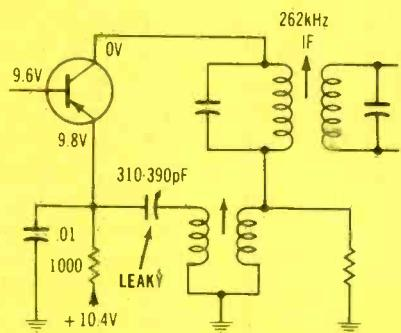
applied to the base, the sound was very weak, but it was loud when touched to the collector. An in-circuit transistor test indicated the transistor was open, and the installation of a replacement restored the proper volume and number of stations.
