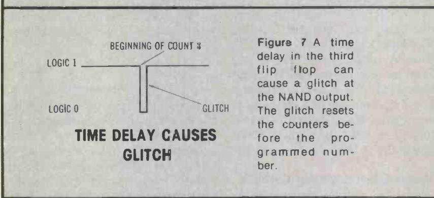
**Figure 7** A time delay in the third flip flop can cause a glitch at the NAND output. The glitch resets the counters before the programmed number.
