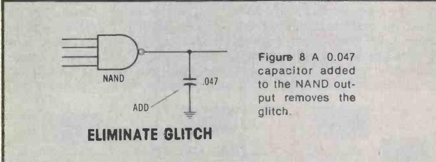
**Figure 8** A 0.047 capacitor added to the NAND output removes the glitch.
