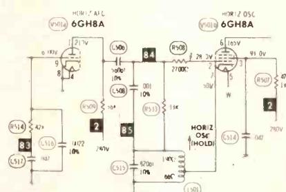
After the TV was brought to the shop, I checked the oscillator and phase-detector voltages. No dc voltage was measured at the plate of V501A (the AFC tube) and R509 checked open. Additional resistance
