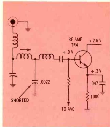
Figure 1 Audiovox model AMF-15 had no AM-band operation.
