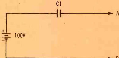
**WHEN CAPACITOR IS UNCHARGED, WHAT VOLTAGE IS BETWEEN A AND B?**
