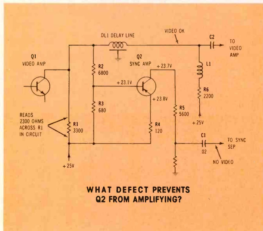
across R1 should have been enough for us (and you) to find the one intermittent component. Notice that not only is R1 paralleled by the sum of R2 and R3, but also R1 is paralleled by R6 (through the delay line and L1). The reading should have been about  $1100\ \Omega$ .
