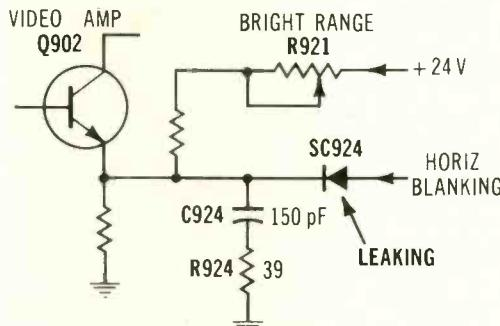
**Symptom**—Horizontal tearing which is changed by brightness
