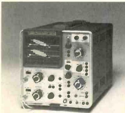
Maximum sensitivity of each vertical channel is 10 mV, and minimum sensitivity is 50 V per division. Bandwidth is from dc to above 15 MHz.
