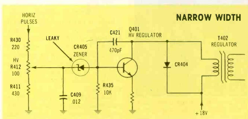
Figure 2 The narrow picture was caused by excessive HV-regulator operation. CR405 leakage forced Q401 to conduct too much saturation current through regulation transformer T402.
