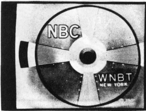
Figure 52—Electrical Horizontal Centering Control Misadjusted
