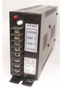
**For most classic games, finding the +5 VDC is fairly easy. If the game uses an arcade switching power supply (like photo to left), just tap onto the +5 VDC terminal of the power supply. Click link above if you need to order an arcade switching power supply.**
