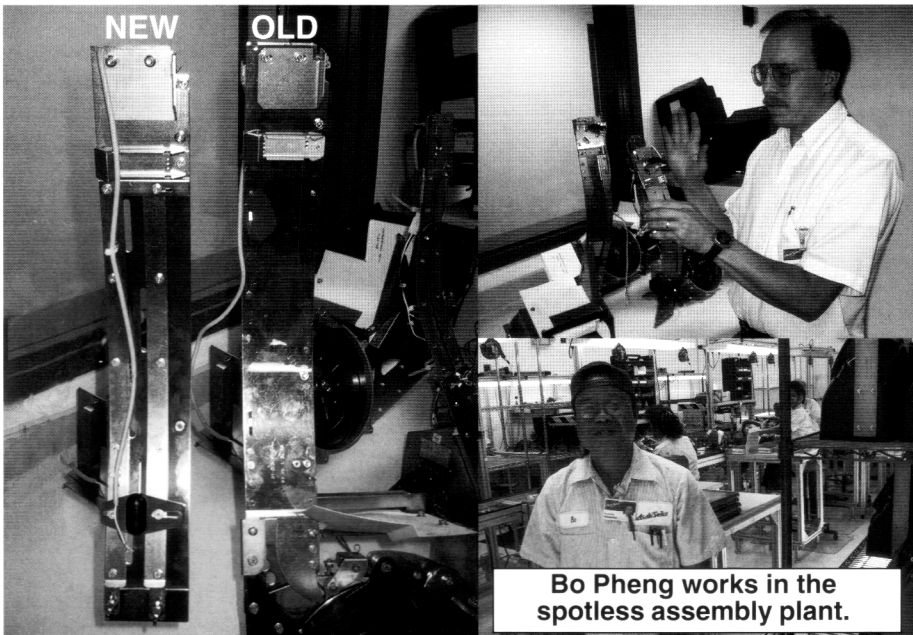
Asahi Seiko engineer Don Seagle discusses their "new & Improved" escalator design, available as a retrofit for Bally hoppers. By inverting the curve, coins travel upward with full support on the backside.
