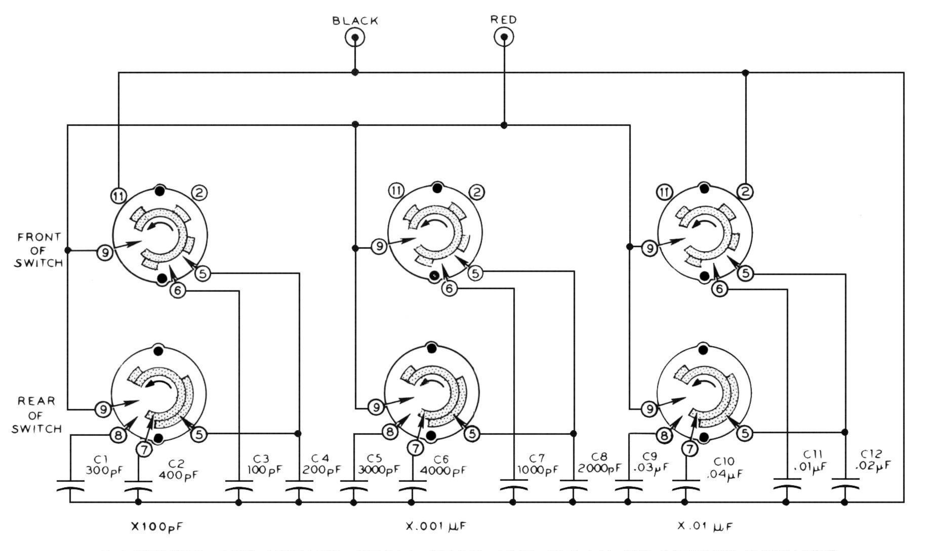
SWITCHES ARE VIEWED FROM REAR AND FULLY COUNTERCLOCKWISE SCHEMATIC OF THE
