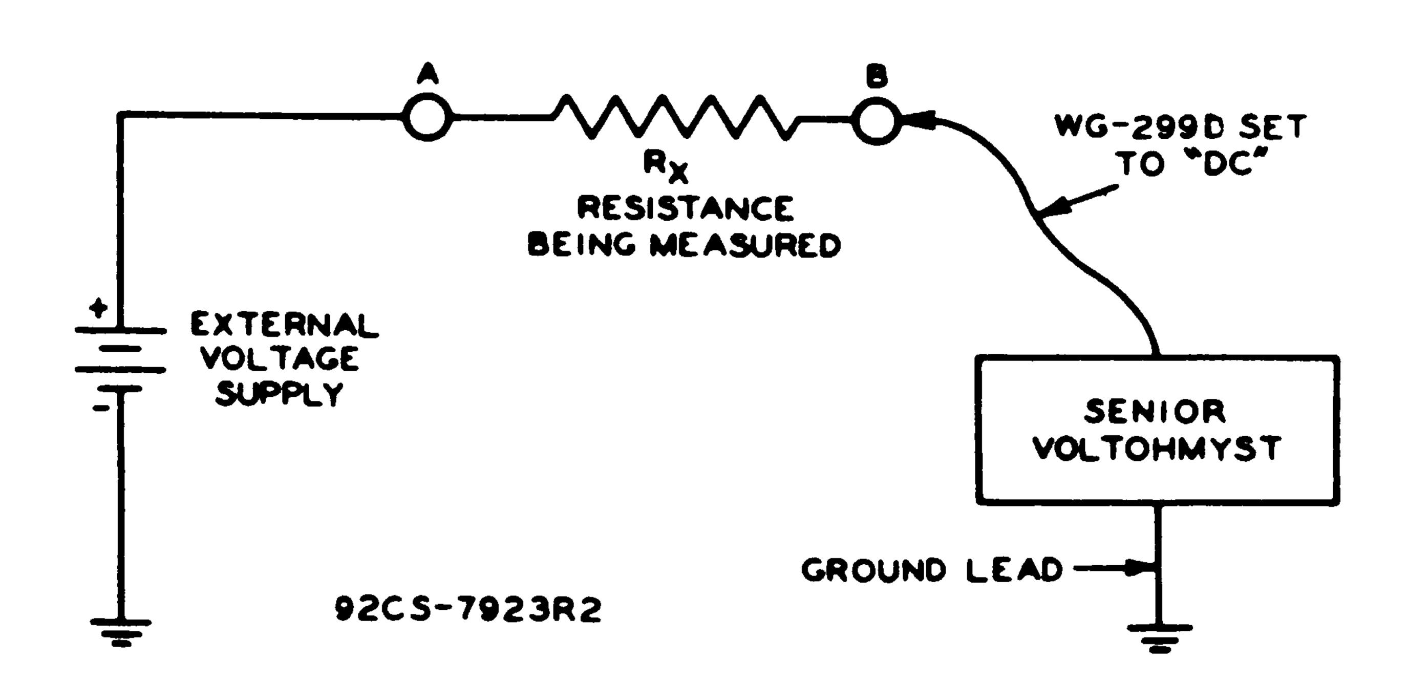
Figure 2. Circuit for resistance measurements above 1000 megohms
