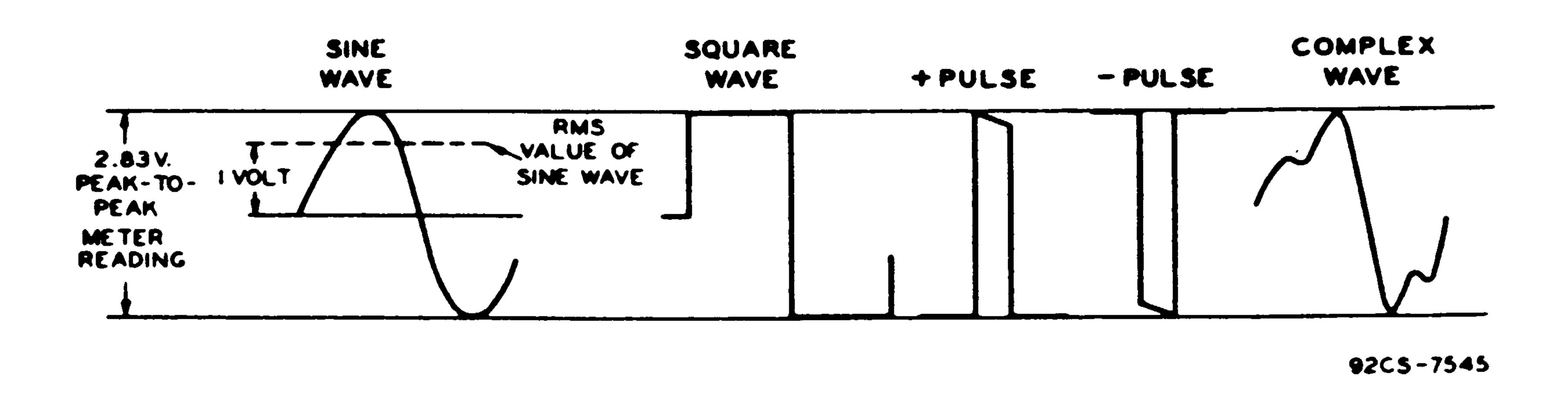
Figure 4. Typical voltage waveforms
