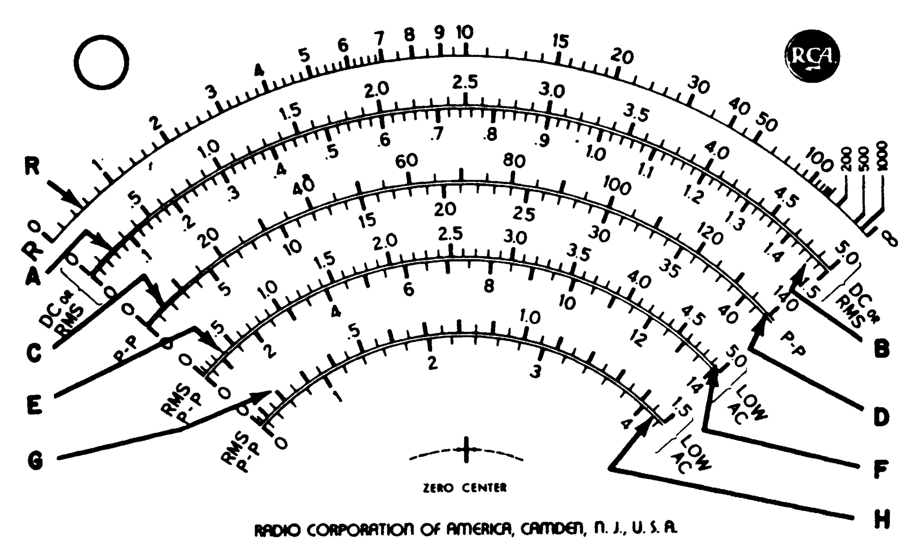
Figure 1. WV-98C meter scales
