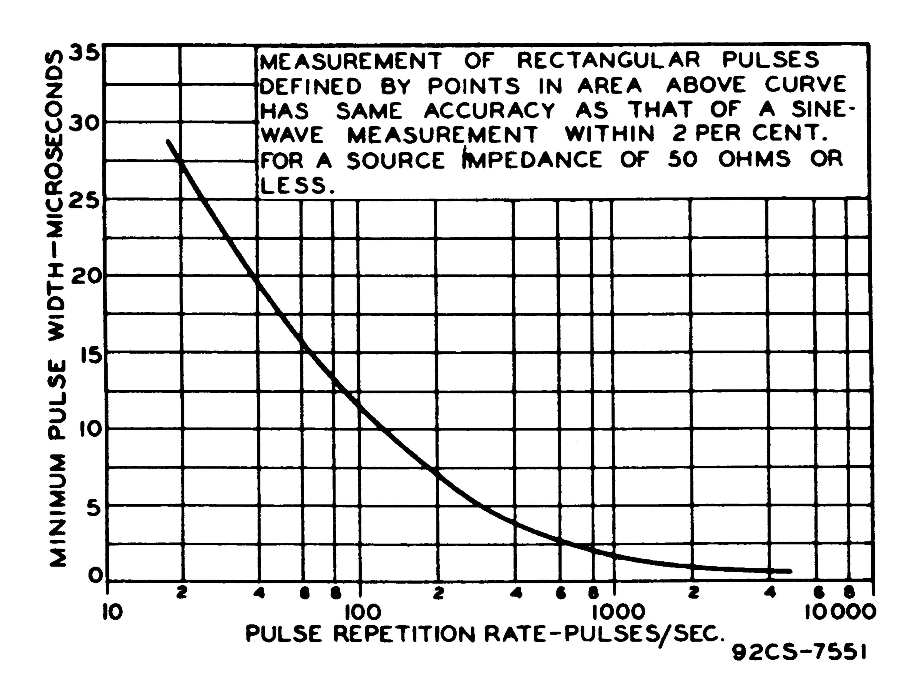
Figure 7. Pulse response capability of the WV-98C
