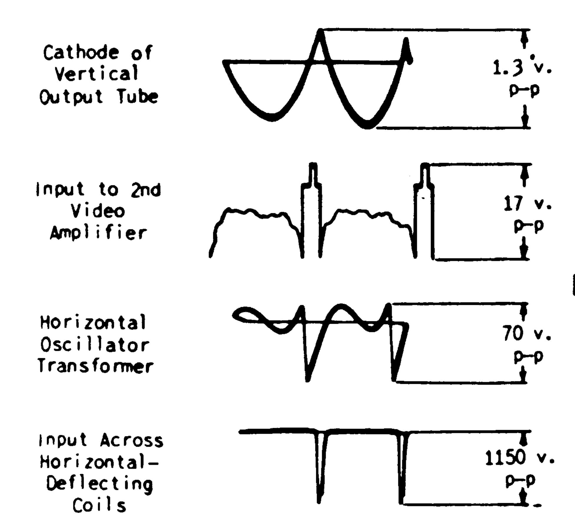
Figure 3. Typical television waveforms
