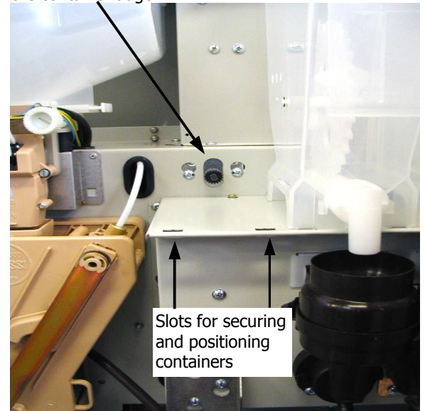
Toothed pinion that drives the container auger
