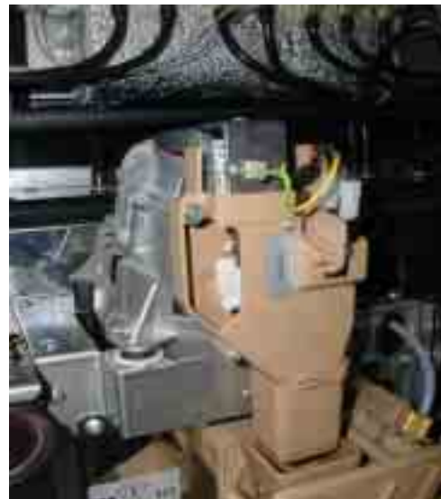
Detail view of grinder doser unit without coffee
